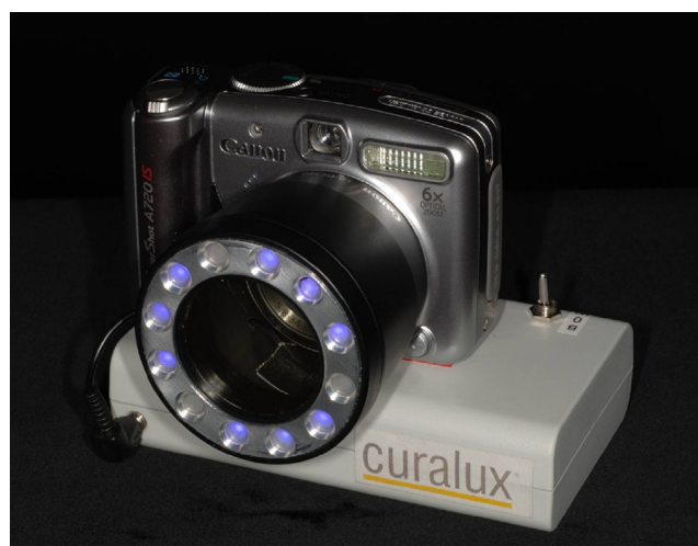
FIGURE 9.2 A portable device for fluorescence imaging incorporating a digital camera, ultraviolet (UV) light source in the form of an LED light, and a power source (Saalmann GmbH, Herford, Germany).
