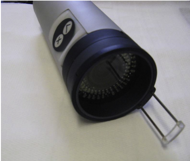
FIGURE 9.4 Handpiece of a dedicated fluorescence imaging device with a stabilizing pod and LED light sources. Photo by author.
