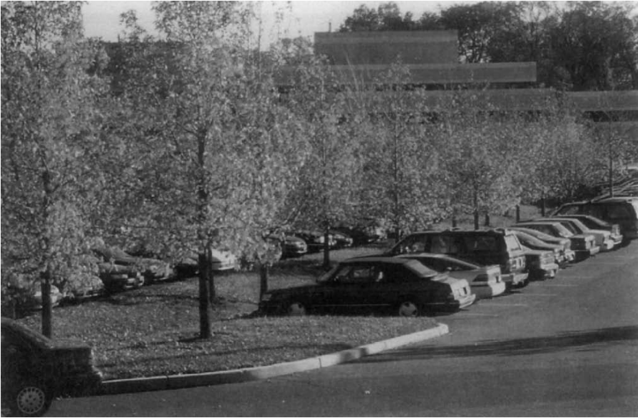
FIGURE 12. The island in this corporate parking lot provides an opportunity for significant tree plantings as well as storm water detention and infiltration.
