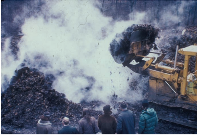
FIGURE 4. Steam released from an oversized pile. (Photo by Franklin B. Flower.)
