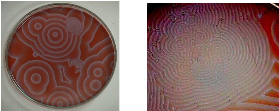
Fig. 12.1 Patterns generated by the reagents of the Belousov-Zhabotinsky reaction taking in a “capsula-Petri”, without stirring. We can recognize target patterns (left), spirals and broken spirals (right). [Courtesy of C. López and E. Hernández-García.]
