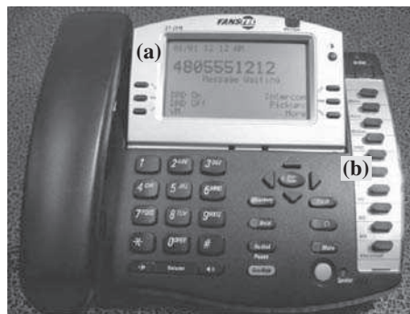
Figure 3.1 ADSI phone: (a) text-based screen; (b) programmable keys (reproduced by permission of © 2008 Fans Telecom Inc. & Fanstel Corporation)
