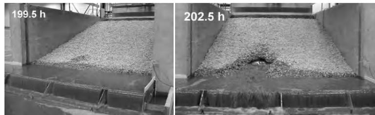
**Figure 2.27.** *Final stage of development of the pipe by perforation of the gravel shoulder*
