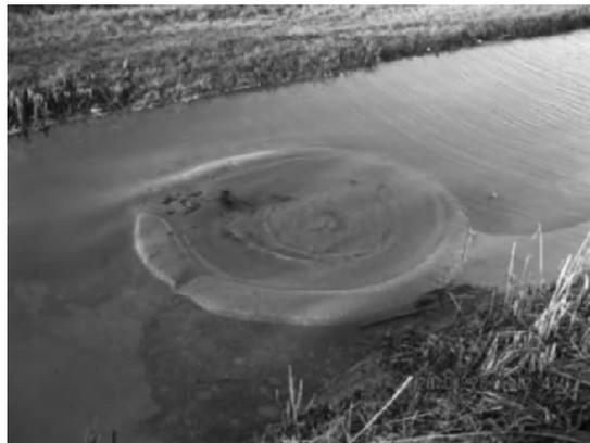
**Figure 3.6.** Sand boil during high water period of 2011 (Hurwenen, The Netherlands)
