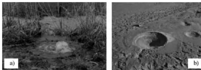
**Figure 3.2.** Sand boil behind a river embankment in a) the Netherlands and in b) France
