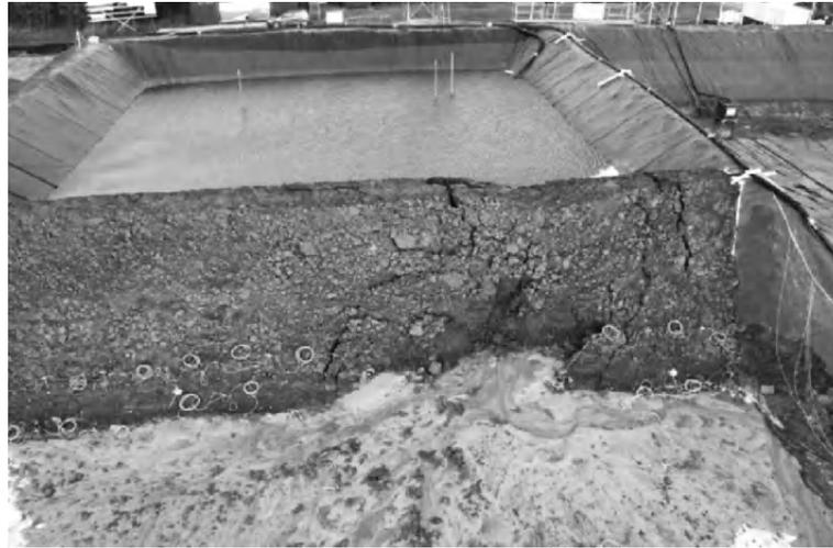
**Figure 3.9.** Failed dike in full-scale experiments [VAN 11]
