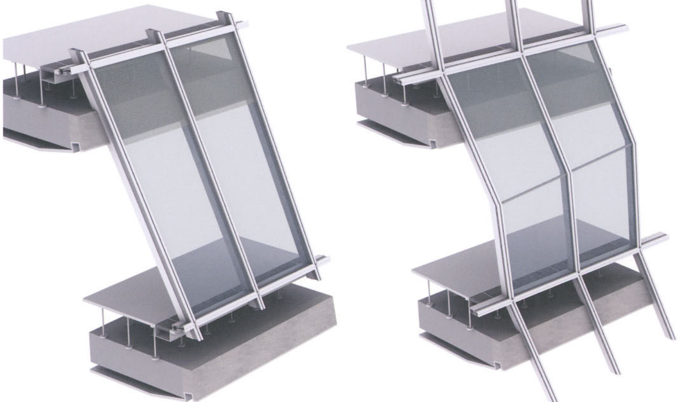
Possible methods of creating a twisted panel using flat glass
