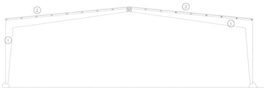
Vertical section 1:100. 3 pin timber frame
