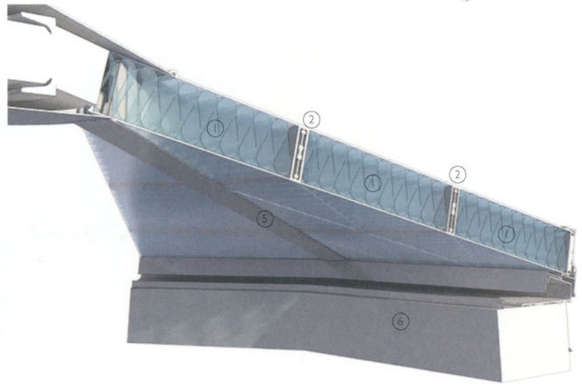
3-D overview of GRP rooflight shell structure
