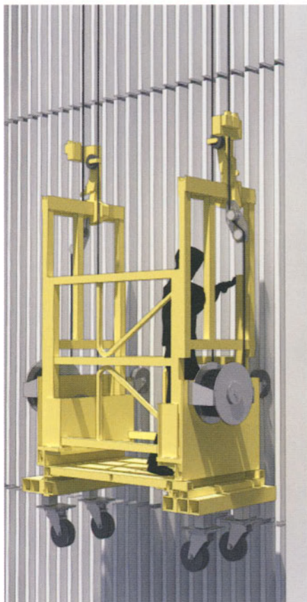
3-D views of typical cleaning cradle on facade
