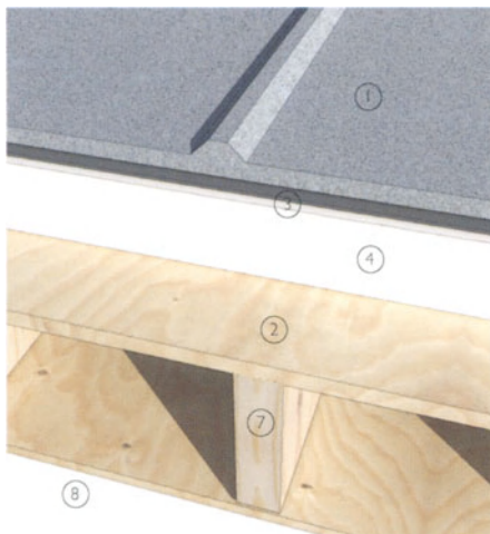
3-D view showing ridge in mastic roof
