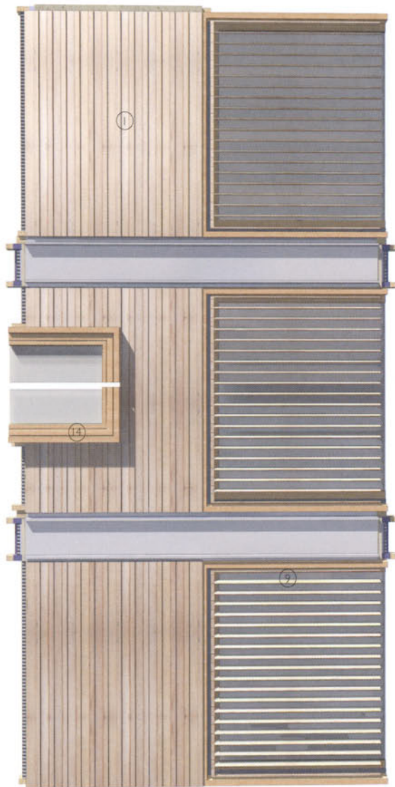
Elevation of timber cladding panels showing relationship with structural frame
