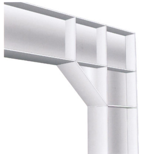
Rigid steel frame corner detail
