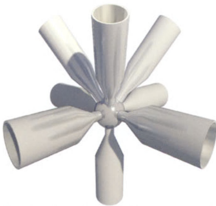
Typical nodes and chords of a space frame structure
