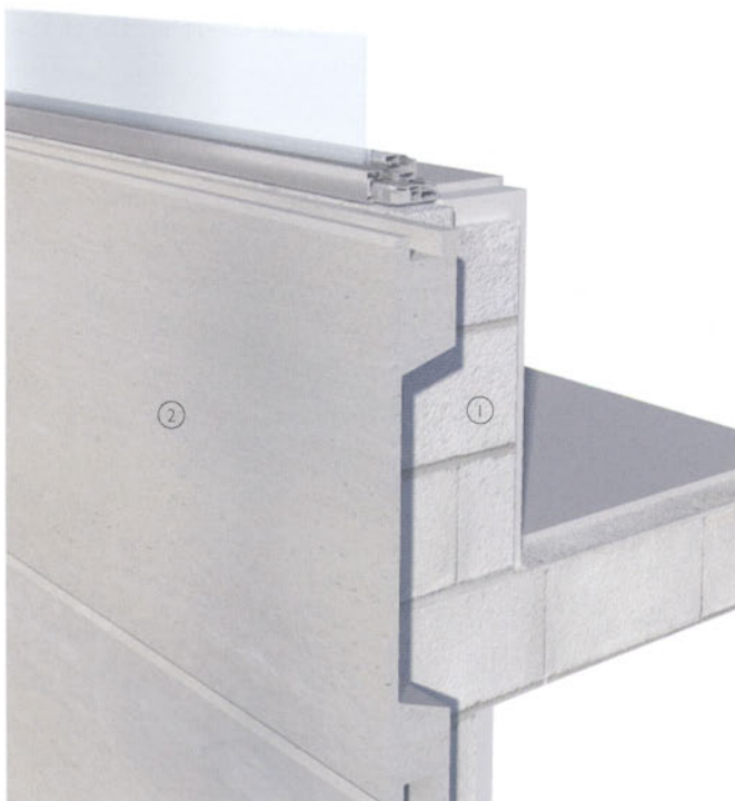
3-D view of wall assembly for GRC panels with open joints
