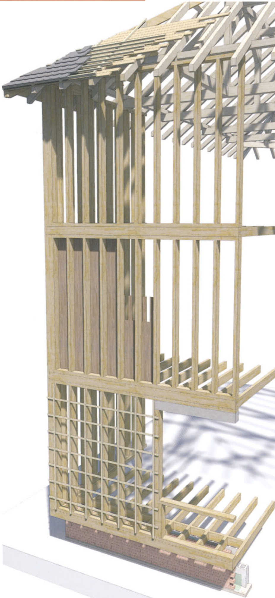
Typical timber balloon frame on a masonry base
