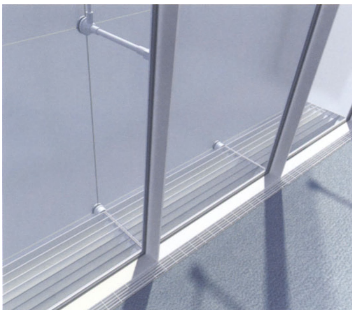
3-D view of twin wall from inside
