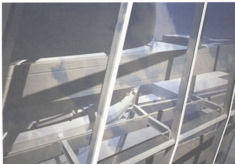
Sectional models explaining the double skin
