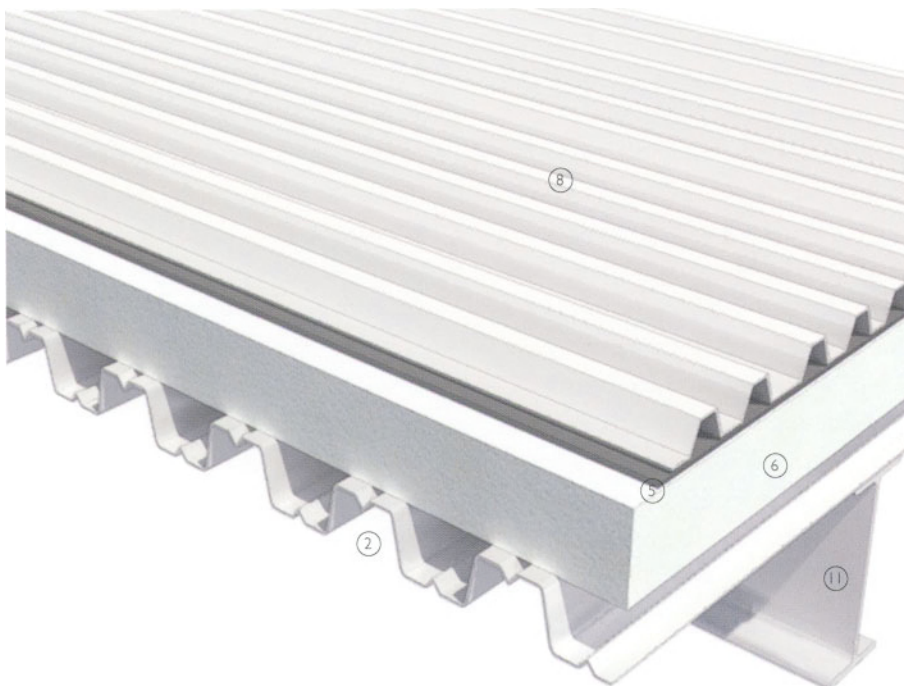
3-D view of profiled metal roof construction
