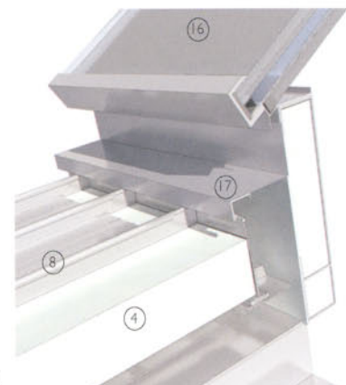
3-D view of metal roof at abutment
