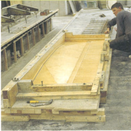
Precast floor components, from timber-based mould to floor panel, beam and panels being installed
