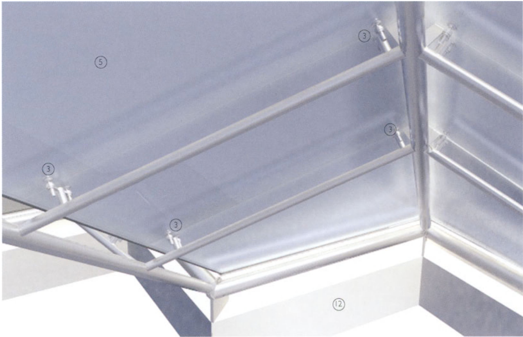
3-D view of underside of bolt glazed roof system
