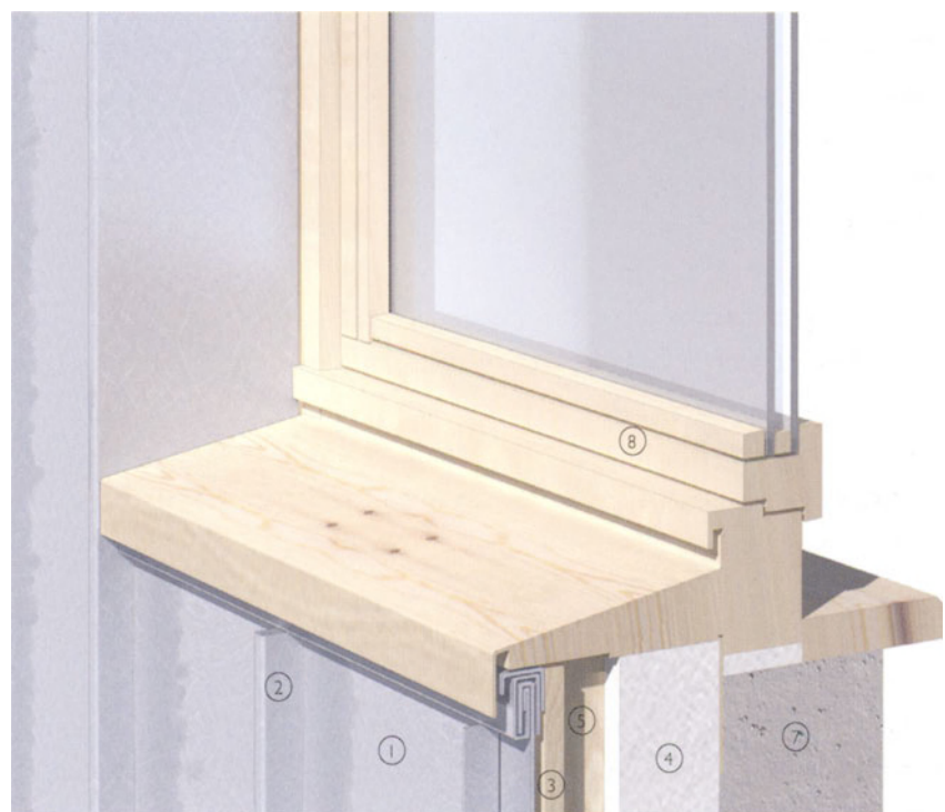
3-D view of window sill detail within profiled metal sheet system
