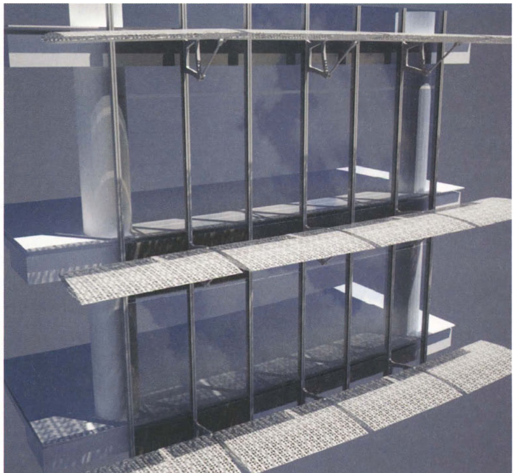
Above and below. Perforated louvers which are moveable allow the shading to track the sun offering maximum protection at different times of day. The horizontal setting shown below would be effective against a high sun whilst the situation above when the sun is lower.
