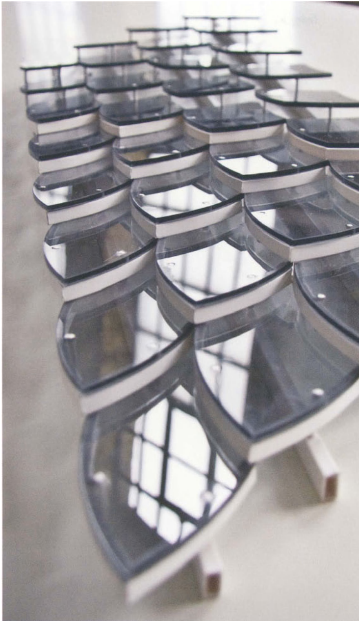
Physical model of facade using pieces laser cut with data exported directly from the computer model
