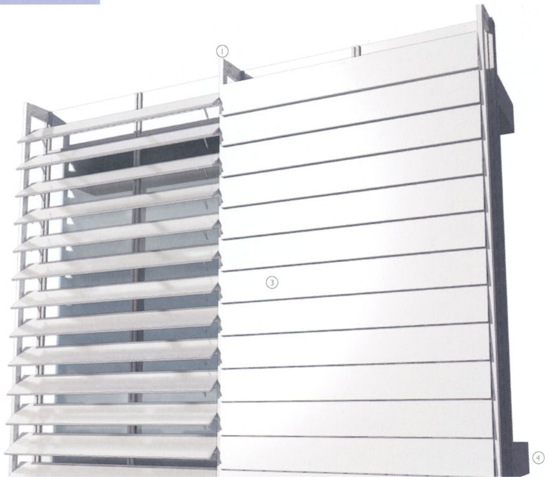
3-D view of metal louvre screen
