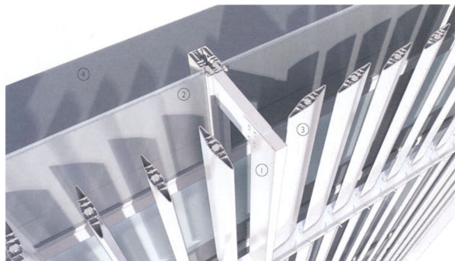
3-D views showing profiled aluminium louvres and fixing system
