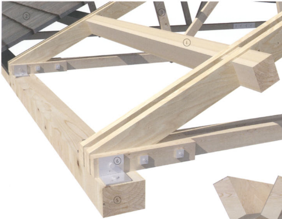
Detail of wall plate connection
