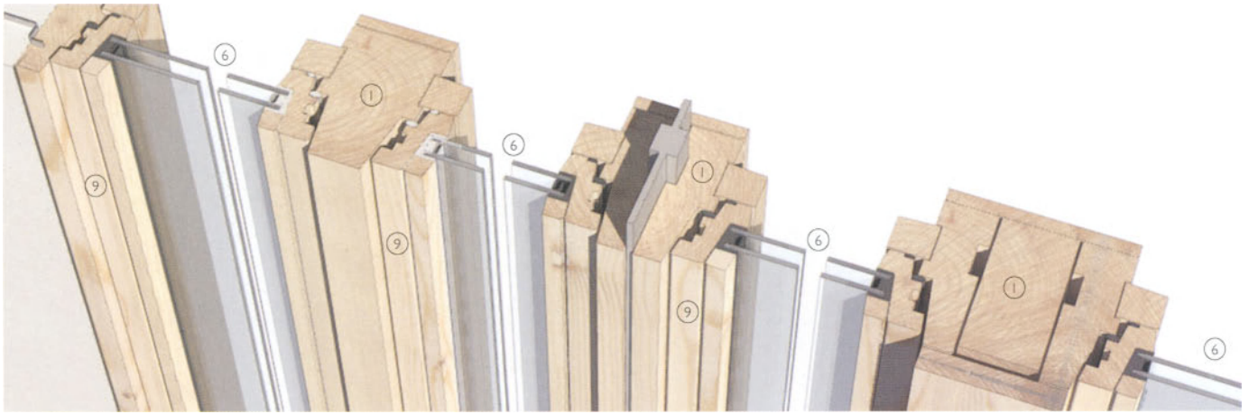
3-D section through side hung window details showing different framing methods
