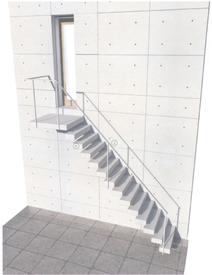
3-D view of cantilevered concrete stair
