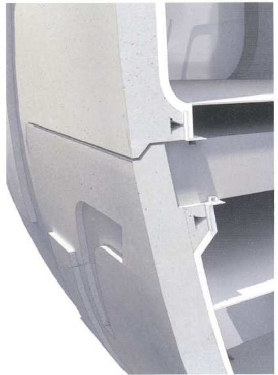
Structural in-situ reinforced concrete backing wall with precast concrete cladding
