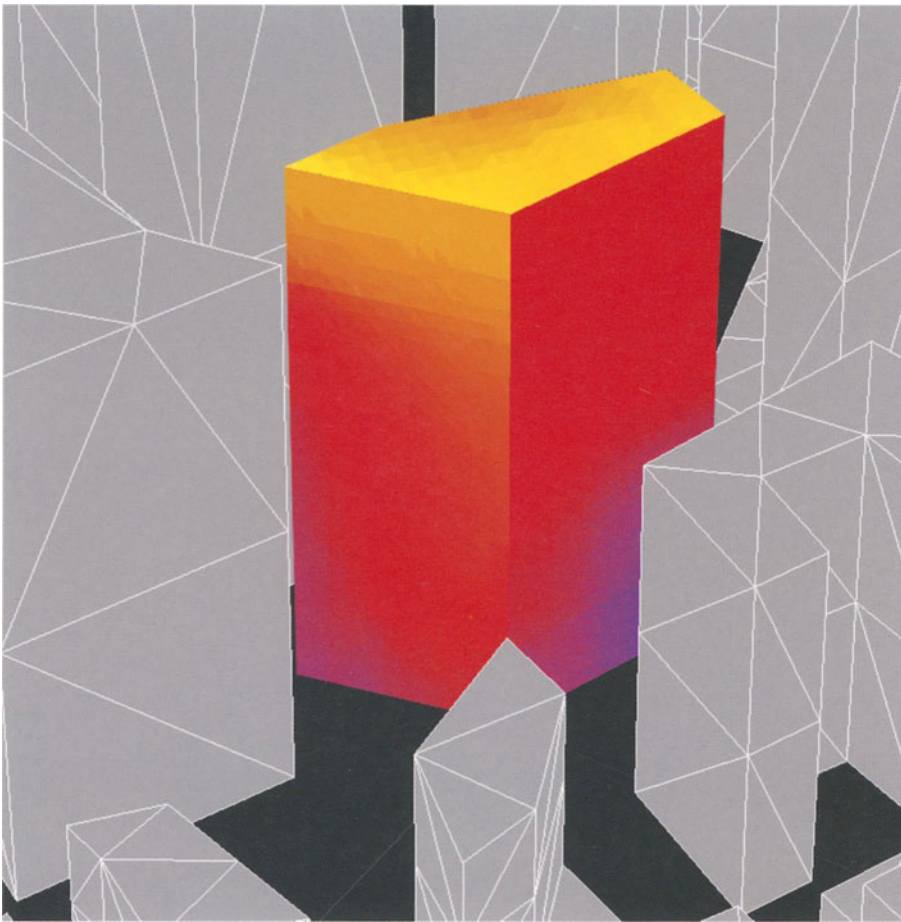
Left: Analysis of the overshadowing effect of surrounding buildings on a proposed facade volume. Areas of the facade closest to the ground are subject to much less direct sunlight
