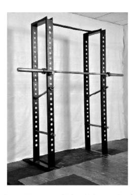
*Figure 8-8.* The best power racks are heavy. This one is welded, and it has uprights of 4-inch channel with holes drilled on 3-inch centers, heavy 1¼-inch pins and chin bar, a heavy plywood floor reinforced with channel, and heavy bolts for hooks.
