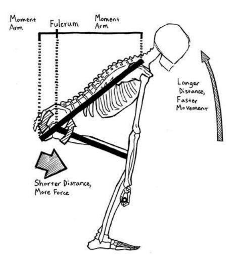
Figure 4-18. The human hip, a Class 1 lever.
