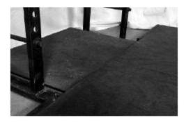
*Figure 8-7.* The rack should have a floor flush with the surface of the platform, so that racking and un-racking weights is safe when trainees are squatting outside the rack.
