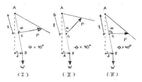
In each of the drawings above the arm hangs at an angle that places the shoulder (point A) a horizontal distance of in front of the weight. The weight pulls downword on the arm at point B with a force W producing a clock-wise moment about point A. The magnitude of this moment is W.d.
