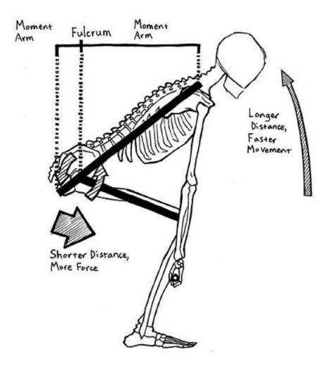
Figure 6-31. The human hip, a Class 1 lever.
