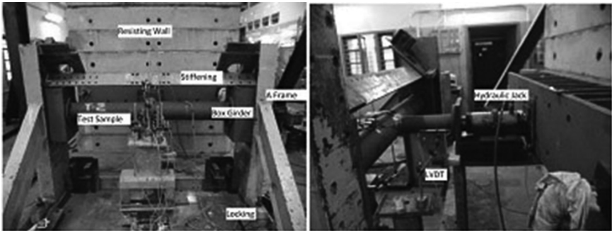
FIGURE 3.19 Experimental setup with components.
