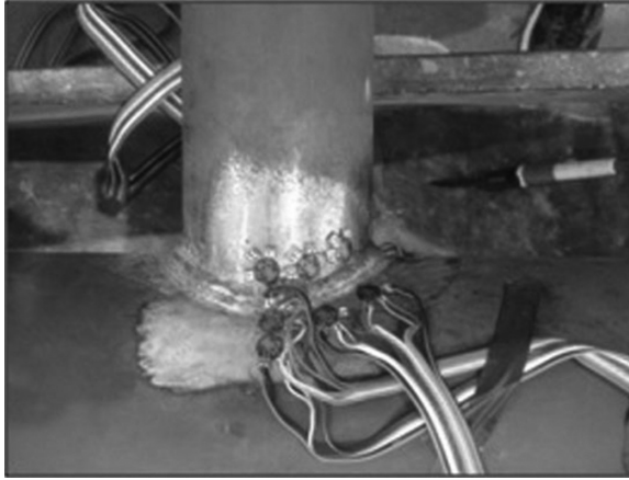
FIGURE 3.20 Sample fixed with strain rosette.
