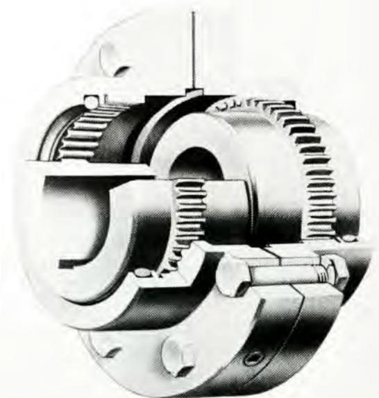
**FIGURE 11-19** Gear coupling. Torque is transmitted between crown-hobbed teeth from the coupling half to the sleeve. The crown shape on the gear teeth permits misalignment. (Emerson Power Transmission Corporation, Ithaca, NY)
