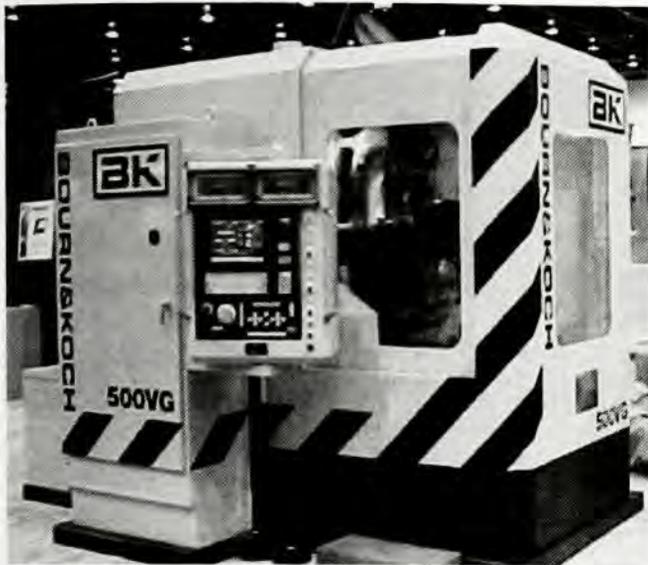
(a) Gear grinding machine
