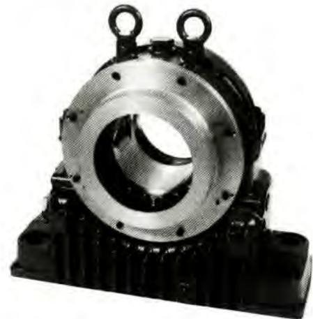
**FIGURE 16-10** Sleevevoil RTL pillow block hydrodynamically lubricated bearing with coolant chambers (Copyright Rockwell Automation/Dodge, Milwaukee, WI. Used by permission.)
