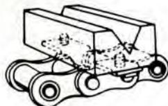
(b) V block assembled to attachments to convey round objects of varying diameters
