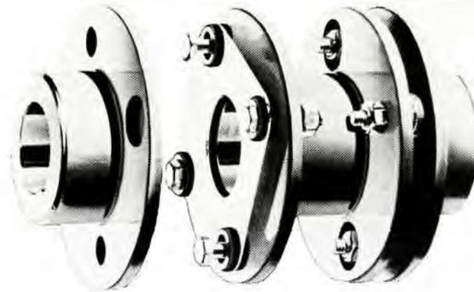
design of the coupling. Small couplings may be limited to parallel misalignment of 0.005 in, although larger couplings may allow 0.030 in or more. Typical allowable angular misalignment is  $\pm 3^\circ$ . Axial movement allowed, sometimes called *end float*, is up to 0.030 in for many types of couplings. (See References 1–3 and the Internet sites for the manufacturers.)
