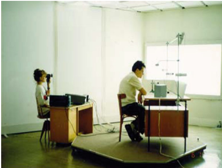
Fig. 12.7 The Slovak Academy of Sciences large-area-source discomfort glare laboratory
