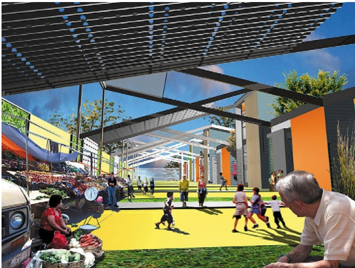
FIGURE 7.18 View of the angular rhythm of rooflines alternating with large open spaces. This arrangement is designed to strengthen the spatial flow among housing units, to provide a flexible climate response of sunlight and shade, and to enhance community-oriented activities like the street market to the left. (Computer model courtesy of Teddy Cruz.)
