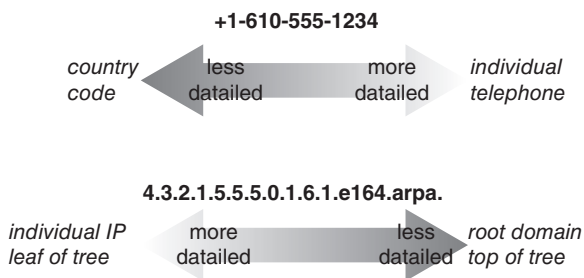
Figure 5-2: Telephone number mapping to domain structure
