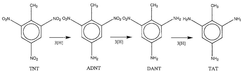
FIG. 7. Anaerobic transformation of TNT.
