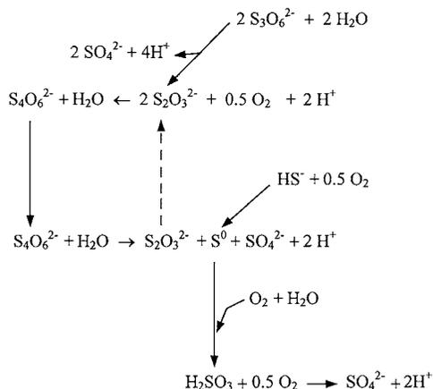
FIG. 7. Schematic diagram showing the sequential reactions during the oxidation of RISCs to sulfate.
