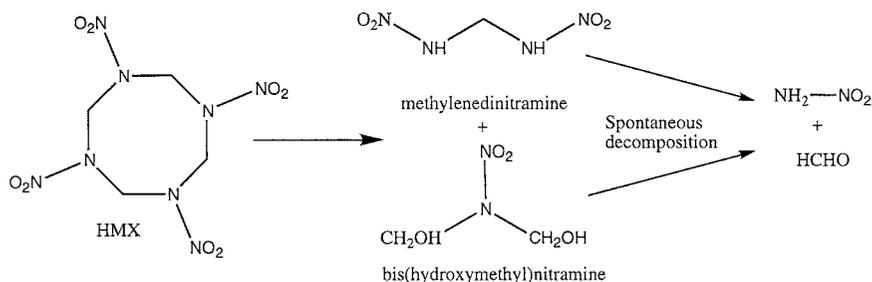
FIG. 11. Ring cleavage of HMX under anaerobic conditions.
