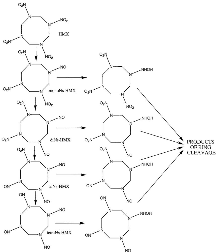
FIG. 10. Sequential reduction of HMX via nitroso derivatives and putative hydroxylamino derivatives.
