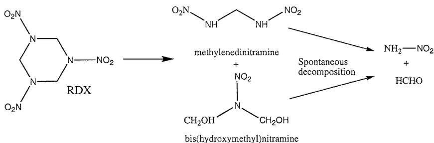
FIG. 9. Ring cleavage of RDX under anaerobic conditions.
