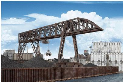
Figure 1.5 A crane truss steel bridge ([paperstreet.iobb.net](http://paperstreet.iobb.net)).
