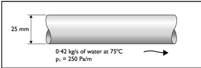
Note that as an alternative approach to step 2, an experienced estimate of pipe size of 25 mm gives a heat loss for uninsulated steel pipe of 92 W/m run (*CIBSE Guide C*, table 3.19), in other words 920 W. This is 5.55 % of the total load, therefore the original assumed loss of 6% is reasonable.
