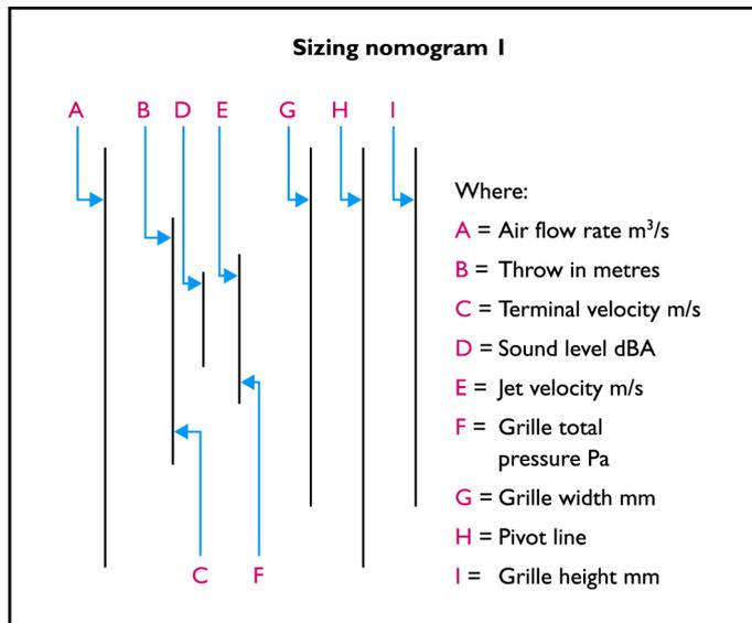
**Step 5. and Step 6.** Plot the required volume flow rate on the appropriate scale on the nomogram (diagram 2).
