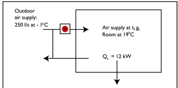
**Step 1.** Supply air temperature and volume - If the outdoor air requirement only were used for heating:
