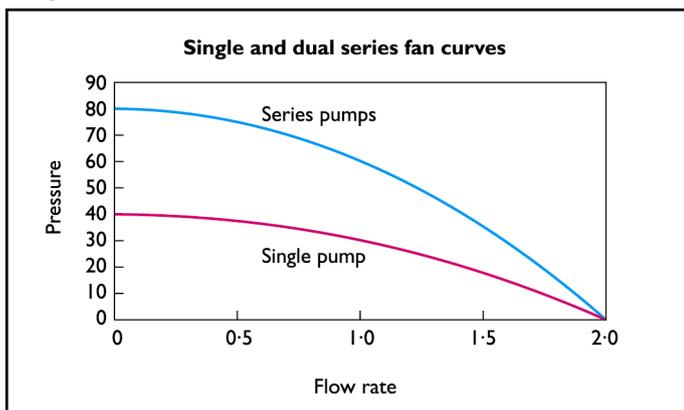
When the system curve is also plotted on the same graph the new operating point can be determined and compared with that of a single pump (see Graph 5).
