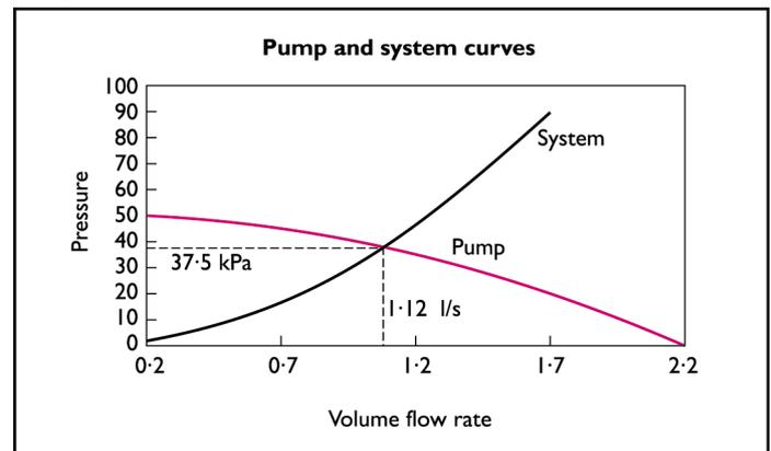
**Step 5.** The operating point occurs when the two curves intersect, 1.12 l/s at 37.5 kPa
