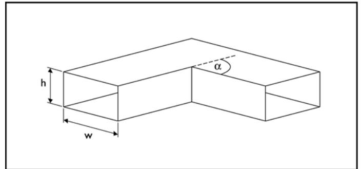
**Step 1.** Height  $h = 0.2 \text{ m}$ , width  $w = 0.2 \text{ m}$ , therefore  $h/w = 0.2/0.2 = 1$  and angle  $\alpha = 90^\circ$ .
