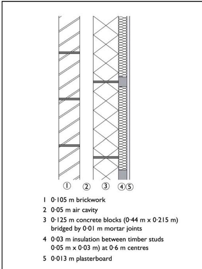
Note: As the thermal conductivities, of brickwork and mortar differ by approximately 0.1  $W/mK$ , the mortar in the brickwork can be ignored in the calculation.
