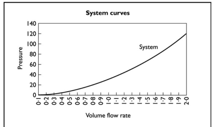
Any system will have a resistance to flow due to the fittings, components, (such as heat exchangers) and the materials used. The flow of fluid through a system will vary according to the pressure developed by the pump.
