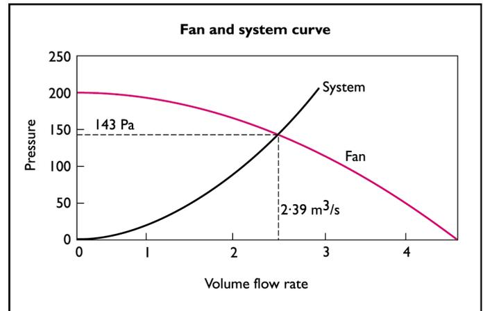
**Step 4.** The operating point occurs when the two curves intersect,  $2.39 \text{ m}^3/\text{s}$  at 143 Pa.
