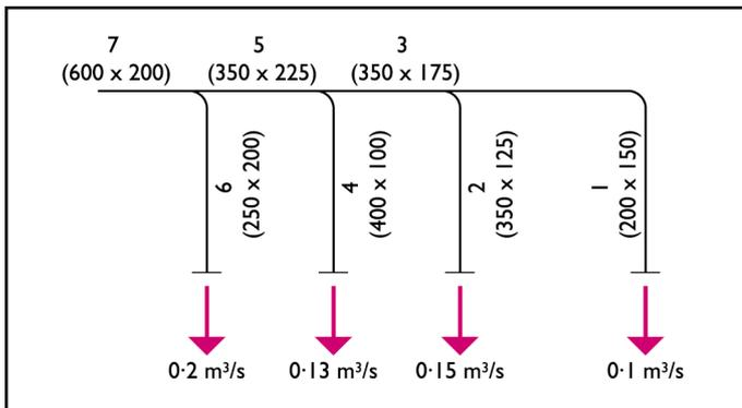
8. It is at this point junior engineers should go back through the duct-sizing procedure remembering to consider dimension ratios, changing one dimension at a time for fittings and the range of standard sizes and costs of using non-standard sizes. A degree of judgement may be required from experienced engineers. The initial dimension above gives awkward changes in dimension, such as  $600 \times 200$  to  $350 \times 225$ .
