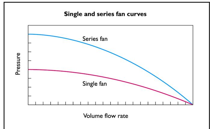
When the system curve is plotted on the same graph the new operating point can be determined and compared with that of a single fan.
