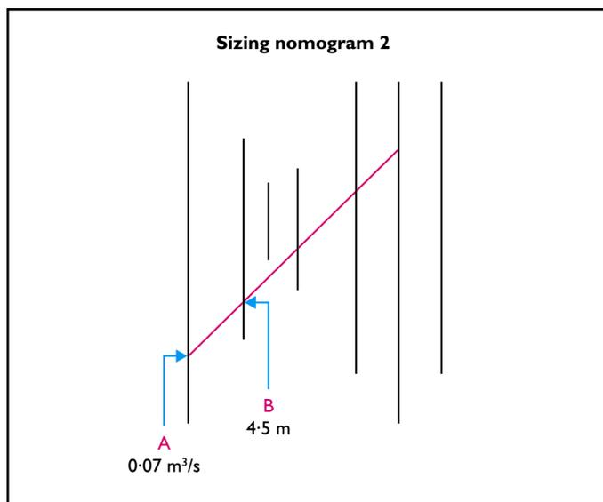
**Step 7.** Draw a line from the selected volume flow rate through the throw point on the appropriate line, (diagram 2), and across to the right hand side of the nomogram. This indicates the following data (diagram 3):
