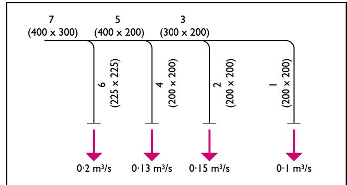
Of course the pressure drops through each section would need to be checked to make sure that they are within acceptable limits for the type of system.
