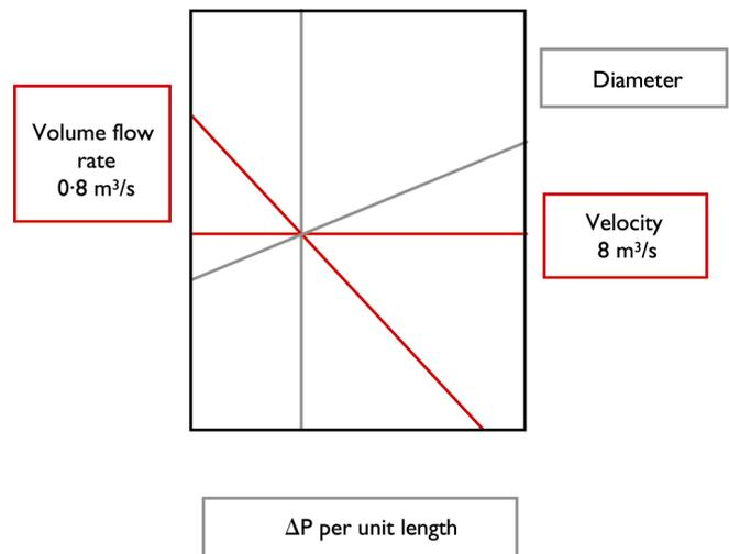
1. Using figure 4.2 *CIBSE Guide C*, draw on the lines that correspond to volume flow rate and velocity, this has been highlighted in red on diagram 3.
