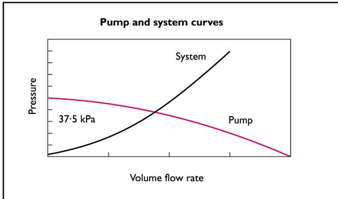
Dual pumps may sometimes be used for various reasons, such as for extra flow or to handle a high system resistance. It may be that the decision to install dual pumps for additional power instead of a single larger pump has been made due to economic costs.
