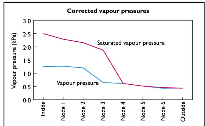
This shows that condensation will not occur anywhere else, as no other nodes have a vapour pressure greater than the saturated vapour pressure. Condensation will only occur where the pink and blue lines meet.
