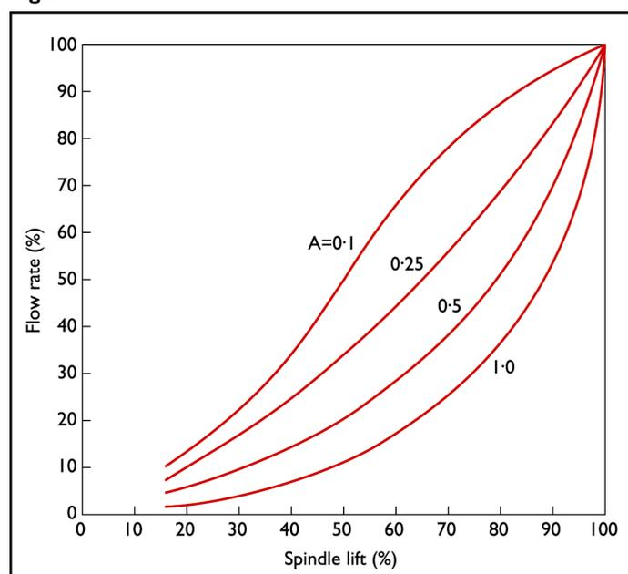
Using Figure 6, these percentage flows can be translated into approximate percentage heat outputs (again for 50 percent spindle lift):
