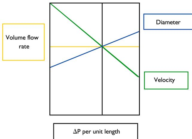
While the volume flow rate ( $q$ ) is usually known from the ventilation requirements and/or heating/cooling loads, one other factor is needed. The second value is either a pre-determined pressure drop per unit length or a pre-determined velocity, (hence the constant pressure drop and velocity methods for duct sizing).
