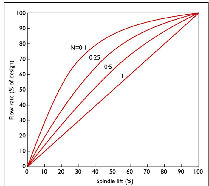
The effect of different valve authorities on the characteristics of an equal percentage valve is shown in Figure 8b of the *ASHRAE Systems and Equipment Handbook*, page 42.8. The curve shown in Figure 5 represents a valve where authority  $N = 1$ .
