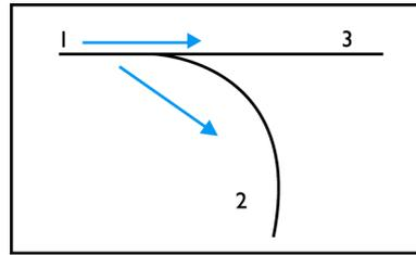
Once the ductwork has been labelled for each section the branch needs to be referenced. The branch fitting consists of two parts, the straight and the branched. The pressure loss for each part will need to be calculated separately as the pressure loss factor ( $\zeta$ ) for the straight length and the branch is often different.
