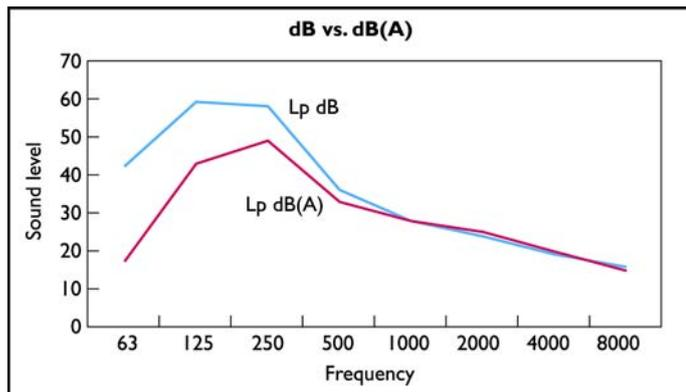
Any sound level given in decibels should indicate whether or not it was weighted when measured and with which set of corrections (in addition to A corrections there are also B and C corrections but these are not covered here). Hence:
