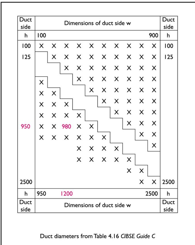
Dimensions given are 1200 mm for side w, and 950 mm for side h.
