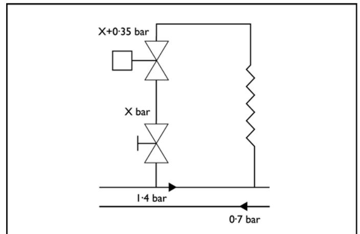
Control valve  $K_v$  for flow of  $2.5 \text{ m}^3/\text{h}$  and pressure drop of 0.35 bar is 4.
