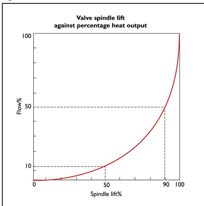
Figure 6 shows the percentage flow against the percentage heat output. The diagram is marked at 10 percent and 50 percent flow giving 50 percent and 90 percent heat output respectively.
