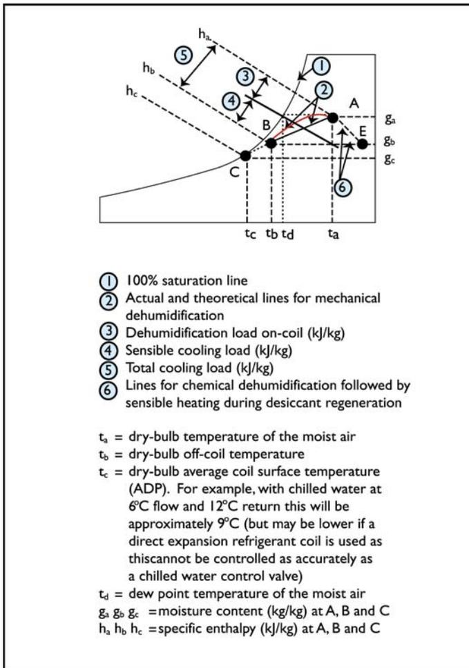
The contact factor is also known as effectiveness. The opposite of the contact factor is the bypass factor. This describes the proportion of air that does not come into physical contact with the coil.
