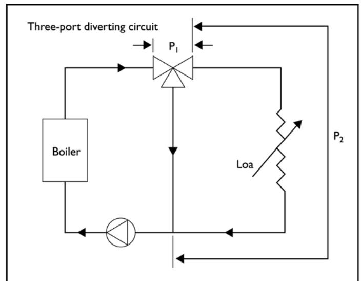
Simple diverting and mixing circuits are shown below, with  $P_1$  and  $P_2$  indicated. Note that these circuits do not show the two-port regulating valves that would be included in the by-pass circuit to make sure that the pressure drop across the by-pass is approximately equal to the pressure drop across the load.
