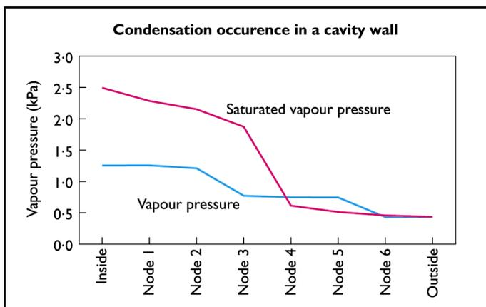
**Step 4.** This shows that condensation will form at nodes 4 and 5 (where the pink line is below the blue on the graph, highlighted in the table). In practice, condensation could begin to form in the insulation near the cavity; this could be a problem. The method must be repeated to check that condensation will not occur elsewhere.
