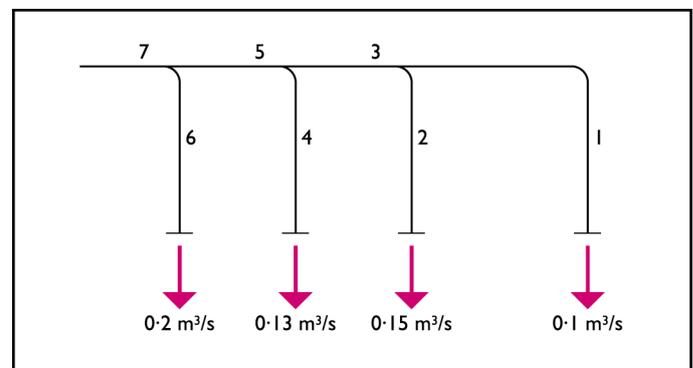
Volume flow rates are worked out for each section and using the *CIBSE* duct sizing chart figure 4.2 the duct diameters and velocities are determined:
