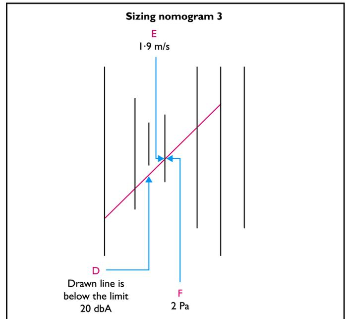
**Step 8.** By rotating about the pivot point, a grille size of  $300 \text{ mm}$  by  $150 \text{ mm}$  has been selected.
