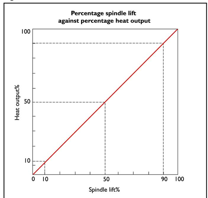
Figures 5, 6 and 7 have been derived on the basis of a constant pressure drop being present across the control valve. In practice this does not happen as the pressure drop across the valve varies depending on how far open or closed it is. The pressure drop is at a maximum when the valve is controlling and at a minimum when it is nearing fully open (*ASHRAE Systems and Equipment Handbook 2004* page 42.8).
