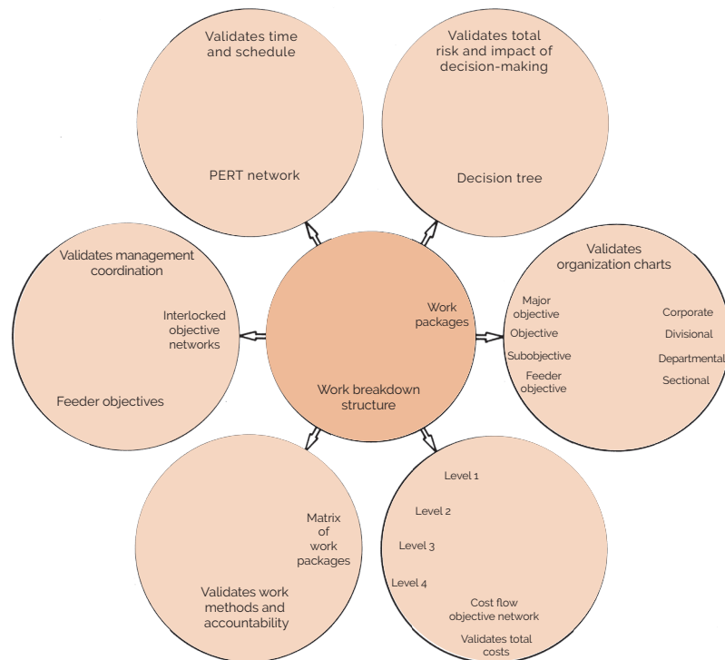
FIGURE 11–2. Work breakdown structure for objective control and evaluation. Source: Paul Mali, Managing by Objectives (New York: John Wiley & Sons, 1972), p. 163. Copyright © 1972 by John Wiley & Sons. Reprinted by permission of the publisher.
