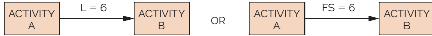
(A) FINISH-TO-START (FS) RELATIONSHIP. THE START OF B MUST LAG 6 DAYS AFTER THE FINISH OF A.
