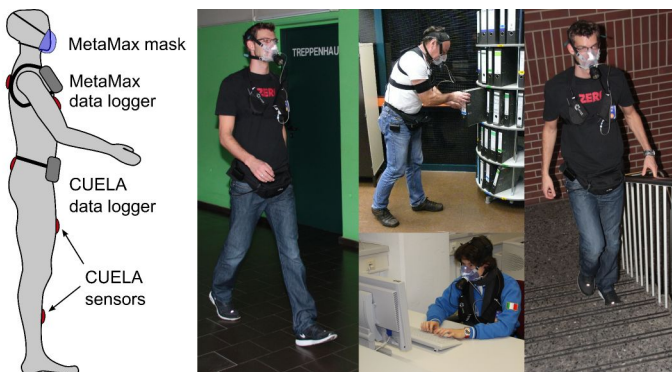
Fig. 1. Measurement instrumentation during activity protocol
