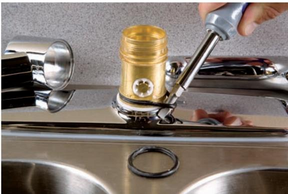
9. Coat the faucet body lightly with silicone grease, and install new O-rings.
