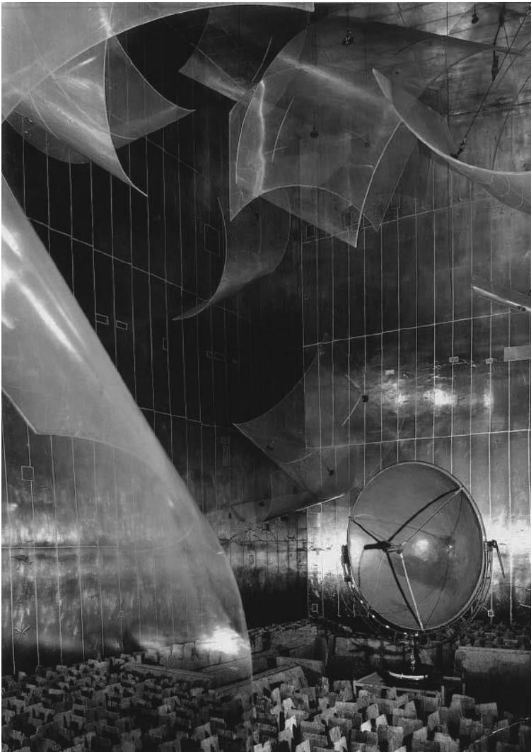
Figure 8.21 Reverberation chamber fitted out with 25 diffusers of Perspex (volume 324 m<sup>3</sup>; dimensions of one shell 1.54 m × 1.28 m).
