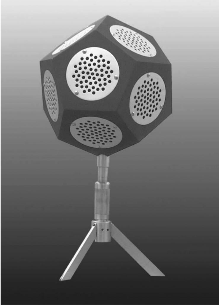
Figure 8.1 Dodecahedron loudspeaker for room acoustical measurements. (Courtesy of Institute of Technical Acoustics, Aachen University, Germany.)
