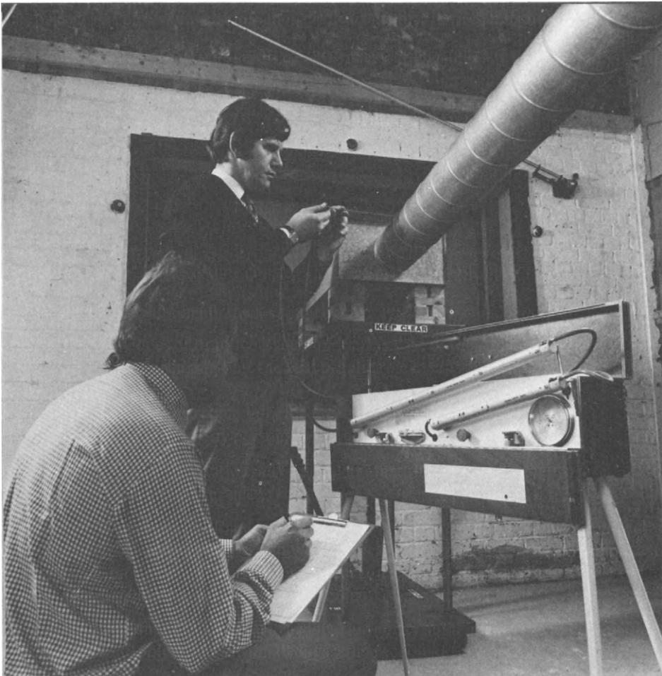
*Figure 13.11b* Air Flow Measurement using a Pitot Travers
