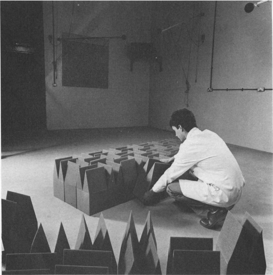
*Figure 13.24* Typical Reverberation Room Test
