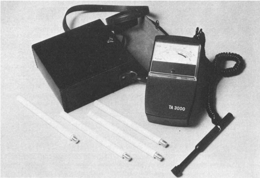
*Figure 13.13* Hot Wire Anemometer
