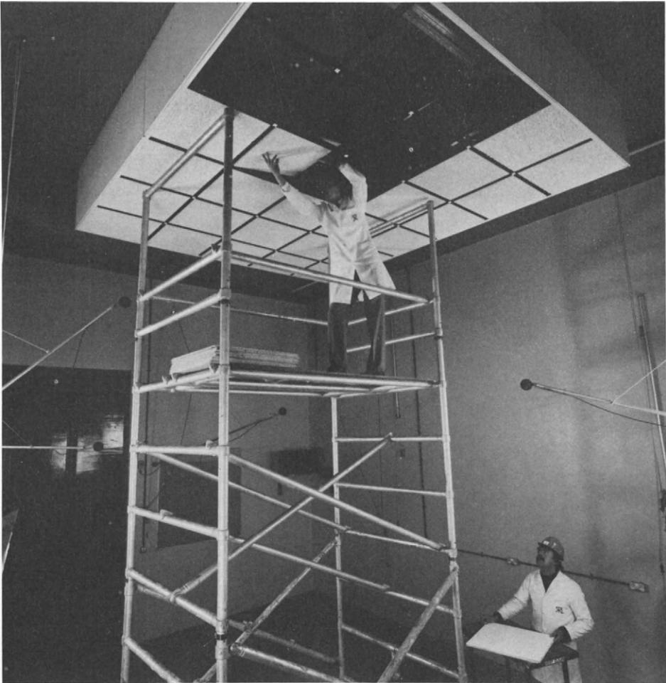
*Figure 13.35* Acoustic Ceiling Tiles being installed for Sound Absorption test
