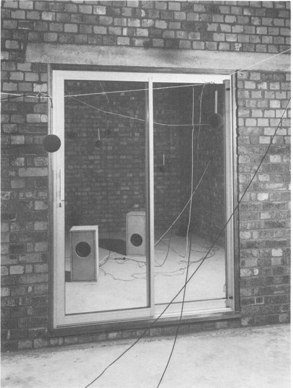
*Figure 13.23 (cont.)* Sliding Patio Doors under test to evaluate their Sound Reduction Index
