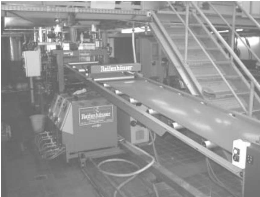
4.15 Extrusion of natural-fibre reinforced PP sheets (source: TITK).
