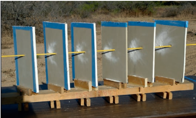
FIGURE 7.5 Bullet perforation of multiple panels of Sheetrock.
