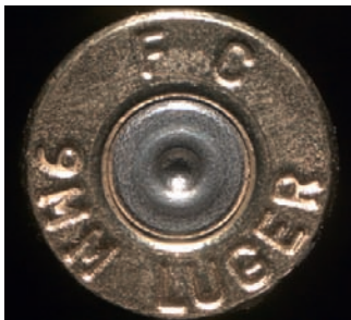
FIGURE 3.6 Second fired cartridge casing showing circular firing pin aperture back flow and a hemispherical firing pin impression. While these class characteristics are relatively common, the arced breech face markings narrow the possible firearm types involved.
