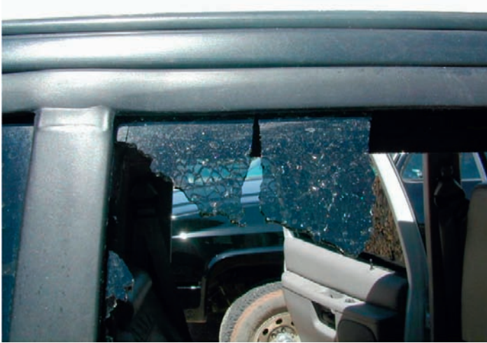
FIGURE 8.16 Diced or broken tempered glass is very fragile; it cannot be driven into the weather stripping if it was previously broken.
