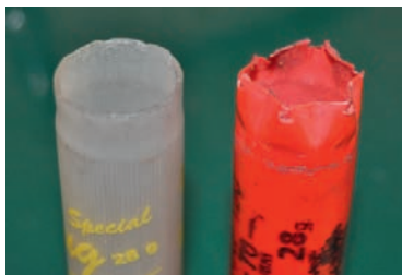
FIGURE 16.4 Two of the most common crimps found on shotgun shells: Roll crimp ( left ) and star crimp ( right ).
