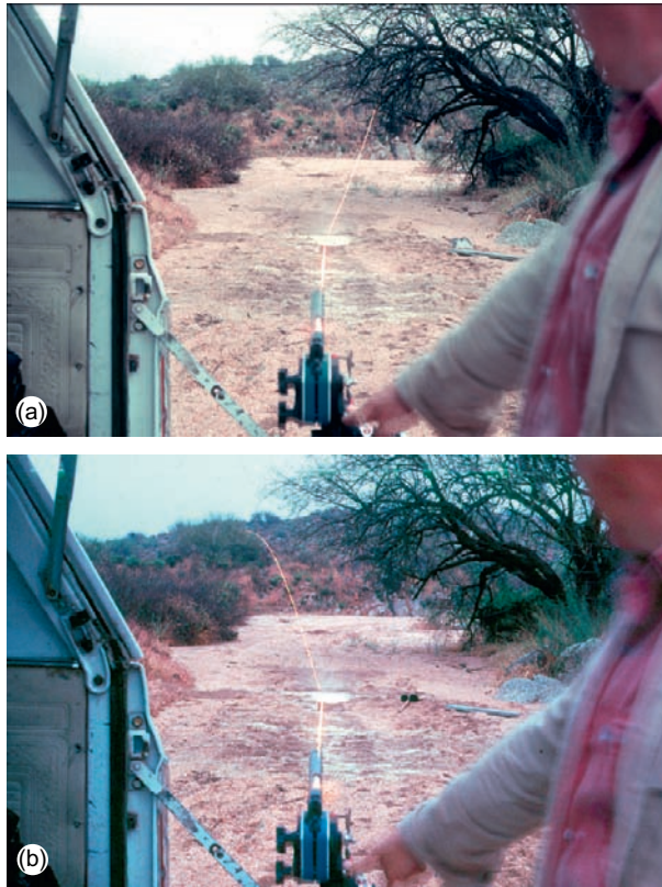
FIGURE 9.5 (a) Over-the-shoulder view of a ricochet from yielding sand, with a right-twist barrel. (b) Over-the-shoulder view of a ricochet from yielding sand, with a left-twist barrel.
