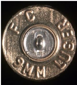
FIGURE 3.5 Fired cartridge casing displaying a rectangular firing pin aperture and an elliptical firing pin impression. Only Glock pistols and early Sigma-style pistols are known to have this set of class characteristics.
