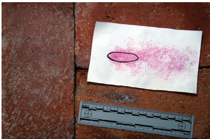
FIGURE 5.5 Lead splash as a result of a low-incident-angle impact and ricochet.
