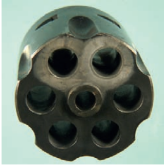
FIGURE 6.8 “Flares” on the face of a cylinder from a revolver.
