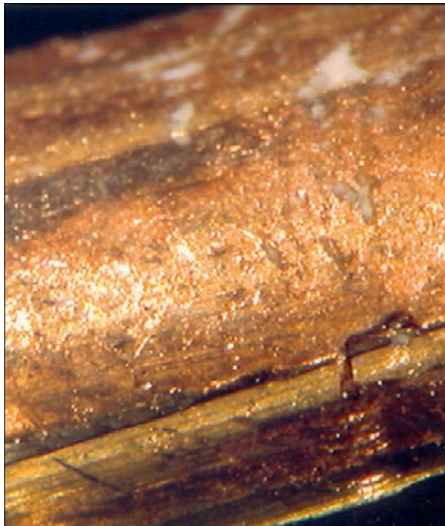
FIGURE 12.3 The entire ogive and the sides of this bullet have glistening embedded glass. In many cases, this can be seen by the trained eye at a shooting scene.
