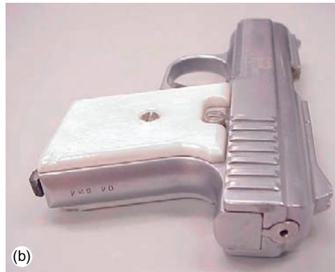
FIGURE 2.21 Here the two images contrast a cocked and ready to fire pistol (a) and one with the striker forward or broken (b).
