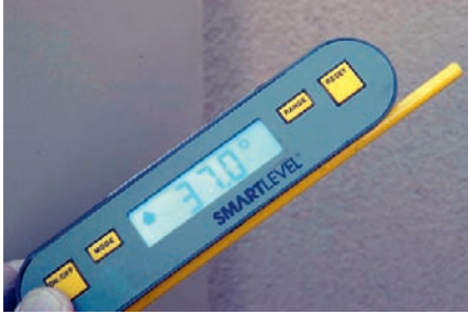
FIGURE 10.3 Vertical angle determination with a digital inclinometer.
