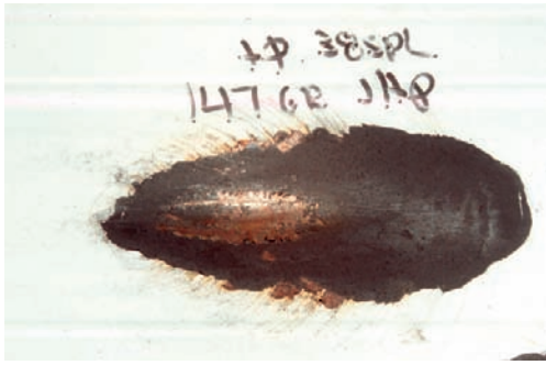
FIGURE 9.17 Fracture lines in paint around a ricochet site in automotive sheet metal.
