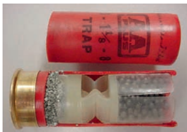
FIGURE 16.2 Sectioned 12-gauge shotgun shell containing #8 shot.
