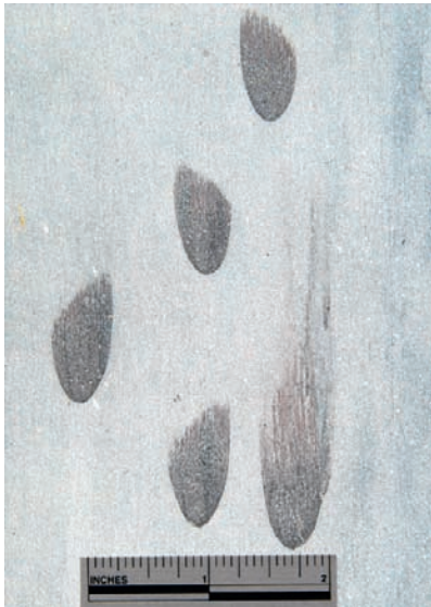
FIGURE 9.8 Diagnostic ricochet marks on hard, unyielding surfaces showing twist direction.
