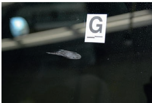
FIGURE 9.3 Example of a pane of tempered glass acting as an unyielding material. Note the parabolic shape on the right side, where the bullet first made contact with the glass.
