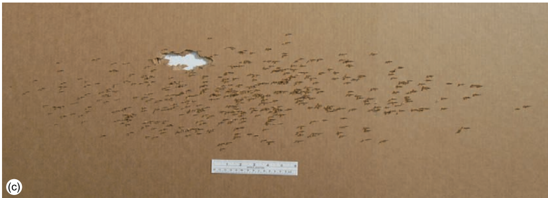
FIGURE 16.17 (a) Orthogonal shot pattern with 6-inch scale in view. (b) A 40-degree angle of intercept shot, with 6-inch scale in view. (c) A 15-degree angle of intercept shot, with 6-inch scale in view.
