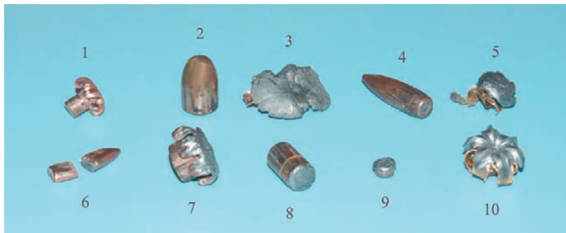
FIGURE 11.4 Assemblage of bullets representing classic forms of “soft” damage.
