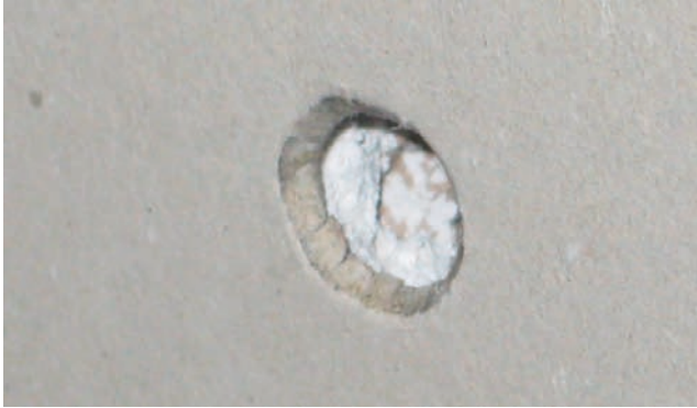
FIGURE 7.3 Basically an orthogonal perforation of drywall by a stable pistol bullet. Note the bullet wipe around the circumference of the hole.
