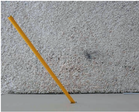
FIGURE 10.4 Photographic method for determining the azimuth component of a trajectory.
