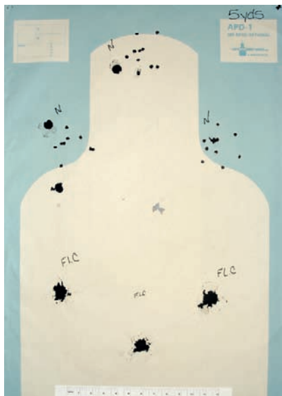
FIGURE 16.13 With a 12-inch scale in view, the difference in pattern size when the distance is kept the same and only the altered ammunition is apparent.
