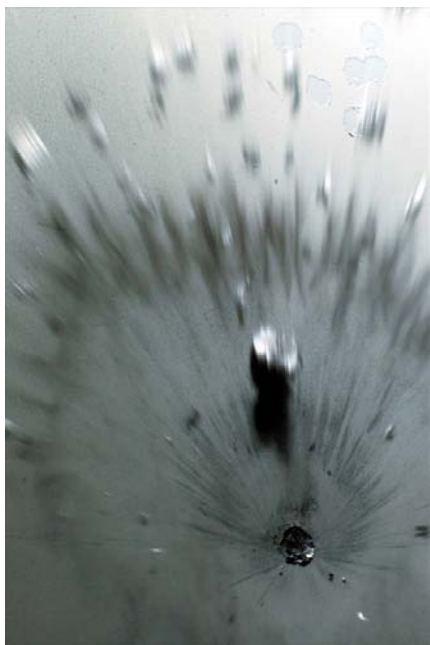
FIGURE 5.4 Example of lead splash.
