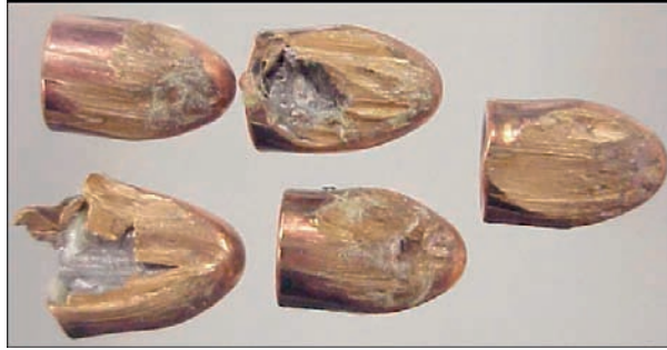
FIGURE 9.14 “Bad” sides of bullets ricocheted from asphalt. The opposite sides are virtually pristine.
