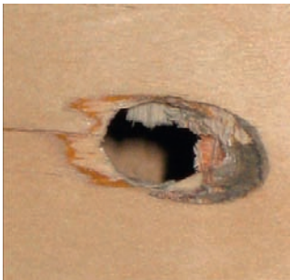
FIGURE 7.7 Oblique-angle perforation of wood.
