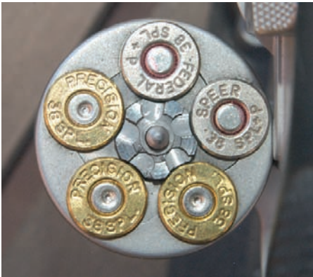
FIGURE 2.9 Next is a close-up of the headstamps and the presence of any firing pin impressions.
