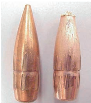
FIGURE 8.2 The effects of glass on a perforating bullet.
