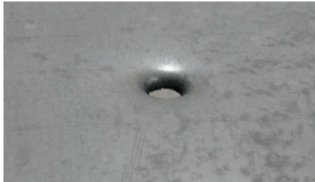
FIGURE 4.3 Deformation typically flows with the direction of travel for malleable materials that deform plastically.
