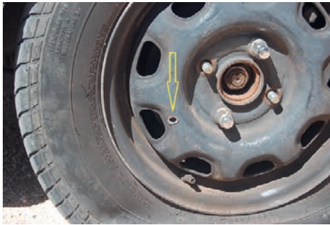
FIGURE 4.8 Counterintuitive entrance of a rifle bullet into a thick, mild steel wheel. A “crown” of metal is visible flowing from the hole.
