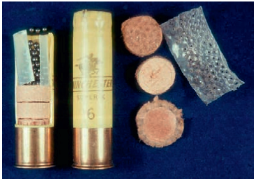
FIGURE 16.1 A 20-gauge shotshell and its fired components.
