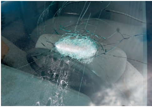
FIGURE 18.7 Nonperforating impact in the windshield of a car.
