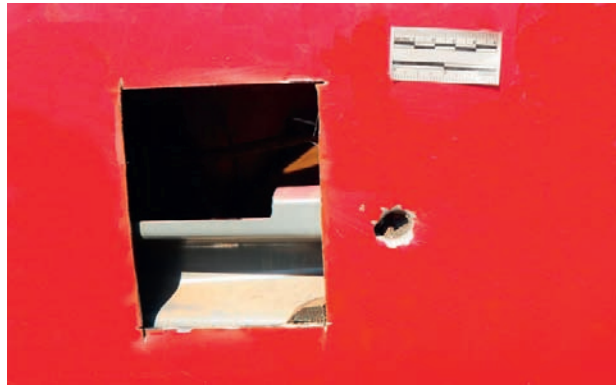
FIGURE 15.6 Primary perforation of the vehicle is the hole to the right of the square viewing window cut out with a cutting wheel. Because the trajectory travels from right to left as viewed, the window allows easy examination of any potential secondary impacts inside the door without altering the original bullet hole.
