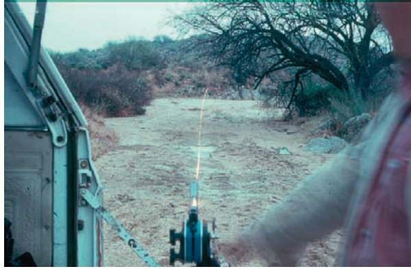
FIGURE 9.4 Over-the-shoulder view of a ricochet from an unyielding stone.
