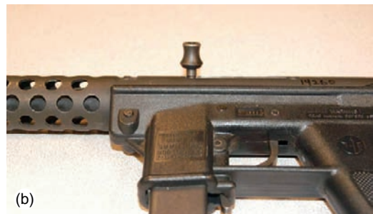
FIGURE 2.22 (a) A gun on safe is shown here and (b) clearly shows the bolt handle further out.
