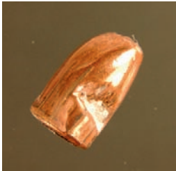
FIGURE 12.2 This bullet ricocheted from wood (note the curved damage to the ogive) and then struck a pane of glass while in yaw.
