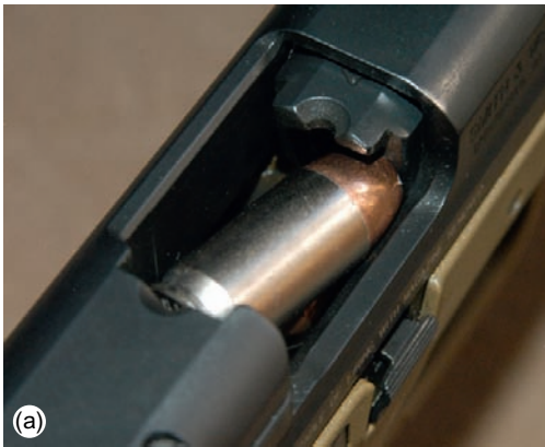
FIGURE 2.16 Here the area of interest is photographed much more closely to show the orientation detail (a) of the jammed cartridge (b).
