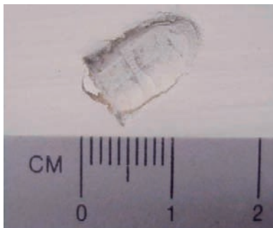
FIGURE 7.1 Bullet impression in painted Sheetrock.
