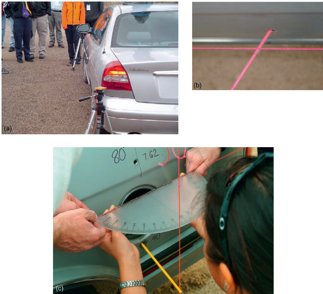
FIGURE 15.1 (a) Two tripods hold taut a string along the side of the vehicle being examined, “squaring” up the curved side into an easily manageable reference line. (b) For azimuth measurements, the crossing of the reference line and trajectory rod is the correct location for a measurement. (c) A plumb bob can be used to efficiently correct for any variation in height between the reference line and the probe.
