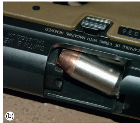
FIGURE 2.16 Here the area of interest is photographed much more closely to show the orientation detail (a) of the jammed cartridge (b).
