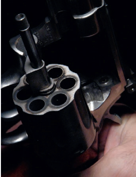
FIGURE 2.1 Front face of the cylinder of a Smith & Wesson revolver. Note the multiple flares, or halos.
