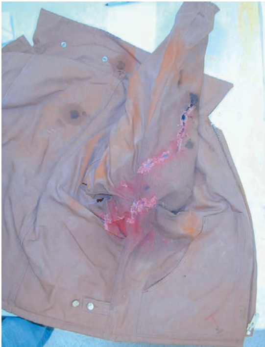
FIGURE 5.9 A light-colored jacket or other garment is a good candidate for the direct-spray method of lead analysis. Rifle bullets in particular will create large amounts of “vaporous” lead as a result of impacts.
