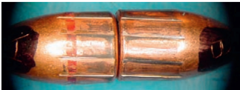
FIGURE 3.12 Two bullets that could have been fired through the same barrel, but comparison microscopy is needed to be certain.
