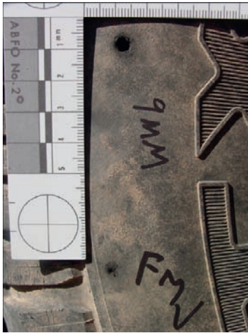
FIGURE 7.16 Two perforations of a rubber tire. While both are the result of a 9 mm Luger caliber bullet, the top hole was created by a hollow-point bullet; the lower, by an FMJ bullet.
