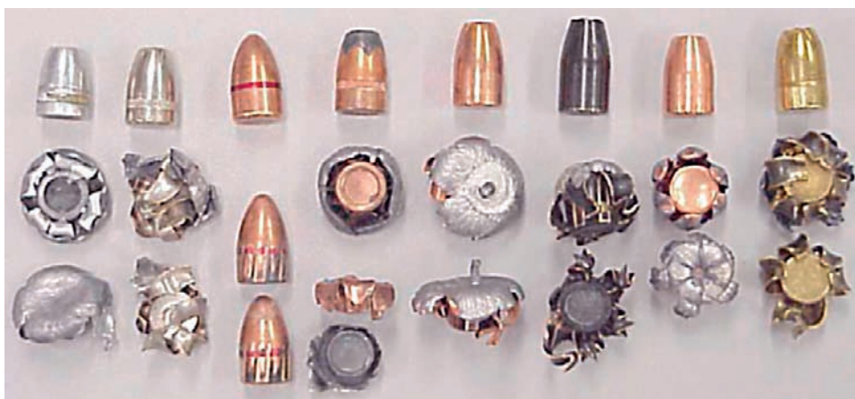
FIGURE 3.2 Selection of bullets from Figure 3.1 after discharge into a tissue simulant. Top row : unfired specimens. Middle and bottom rows : two examples and views of each bullet after discharge. Note the unique, surviving characteristics of many of these bullets.
