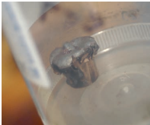
FIGURE 3.4 Federal Hydra-Shok bullet. As with many higher-end bullets, there are distinct and unique manufacturing characteristics to be seen. Here, the telltale lead post emerges from the mushroomed nose.
