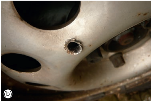
FIGURE 7.19(B) “Crown” effect at the entrance of a 223 caliber rifle bullet at a relatively thick, mild steel wheel. Intuitively, the image in (a) seems more like an exit than does the image in (b).
