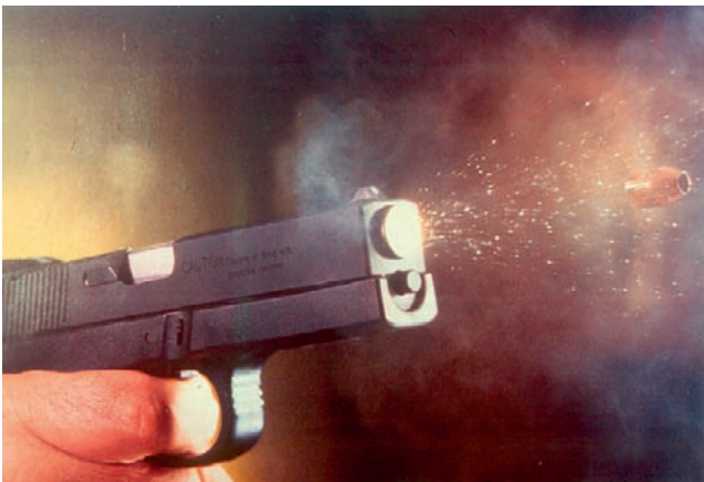
FIGURE 3.13 Gunshot residue production from a semiautomatic pistol.
