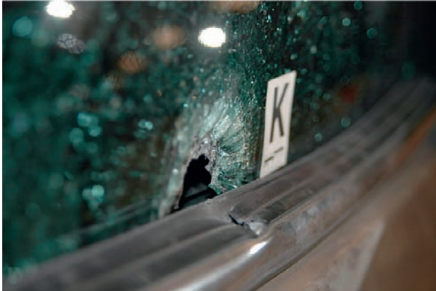
FIGURE 8.15 Beveled, primary defeat of a pane of tempered glass as viewed from outside the vehicle.
