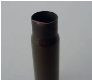
FIGURE 14.1 Red paint on the mouth of a 7.62 × 39 mm cartridge casing.
