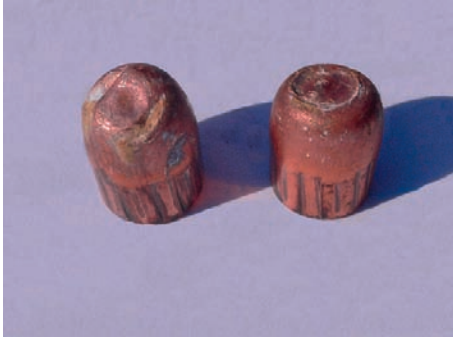
FIGURE 12.2 This bullet ricocheted from wood (note the curved damage to the ogive) and then struck a pane of glass while in yaw.
