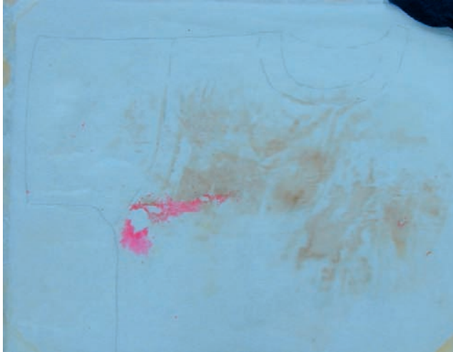
FIGURE 5.11 Reverse image of a sodium rhodizonate lift of the T-shirt shown in Figure 5.10. One of the lift technique's best properties is its ability to show pattern information for lead deposits where they may not have otherwise been visible. Note the reference lines drawn from the T-shirt.
