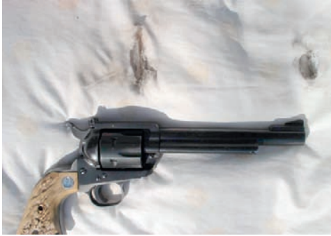
FIGURE 17.14 A pillow and gun after the discharge of a Ruger Blackhawk. Note the obvious barrel length relationship between the cylinder gap deposits and damage and the muzzle deposits and entry hole.
