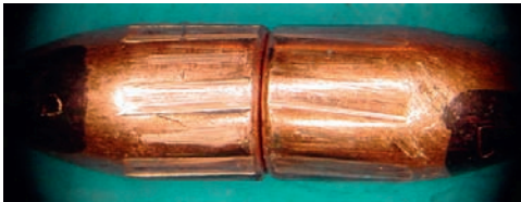
FIGURE 3.10 Two bullets of the same caliber, with the same number of lands and grooves but with differing direction-of-twist rifling. These bullets must have been fired through two different barrels.
