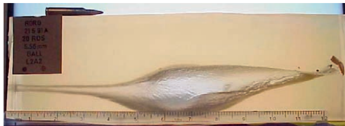
FIGURE 11.2 Path of an unstable bullet in a tissue simulant.
