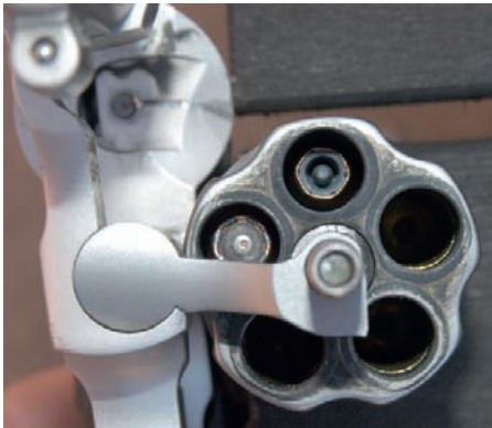
FIGURE 2.10 One or more photographs showing the front of the cylinder captures the presence of any flares/halos, and potentially the types of projectiles loaded in the cartridges.
