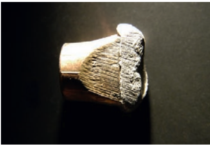
FIGURE 9.10 Important features include unyielding material impact damage, impact striae that traverse the bullet off angle from the long axis, a lack of trace carpet fibers in the nose, and a minimal amount of expansion.
