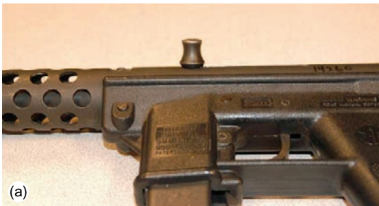
FIGURE 2.22 (a) A gun on safe is shown here and (b) clearly shows the bolt handle further out.
