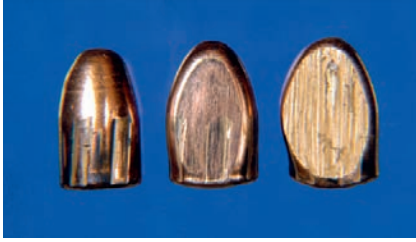
FIGURE 9.6 Bullets ricocheted from smooth concrete and polished granite.
