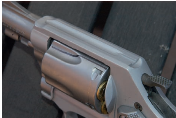
FIGURE 2.7 For revolvers, scribe the cylinder with a permanent marker on both sides of the top strap to show its orientation before opening.
