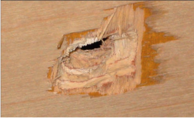
FIGURE 7.8 Exit corresponding to the perforation shown in Figure 7.7.
