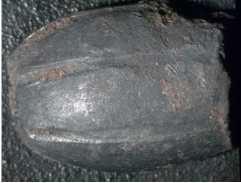
FIGURE 3.3 Lead Federal Hi-Shok bullet core. The nose is to the left; the base, to the right as viewed. Raised ribs on the inside of the jacket create the furrows in the lead core.
