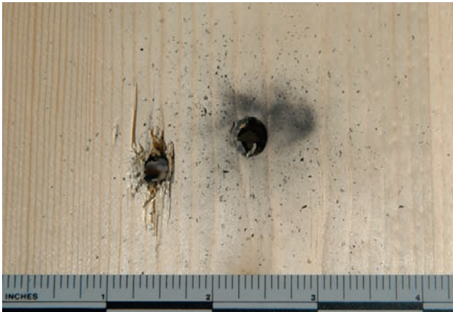
FIGURE 6.3 Gunshot/residue/powder pattern on wood.
