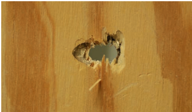
FIGURE 4.2 Entrance hole in plywood. Note the parabolic shape on the left side and the lead-in mark or partial bullet wipe on the acute side of the impact.
