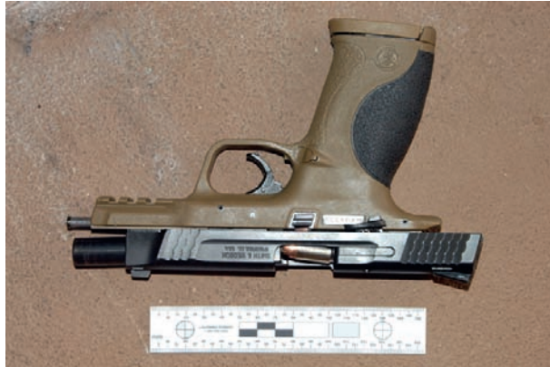
FIGURE 2.15 Photograph of the pistol after being flipped over carefully, and in this case, a failure to feed is exposed.
