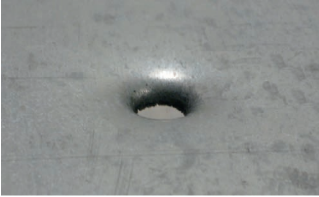
FIGURE 7.11 Orthogonal perforation of a piece of sheet metal.
