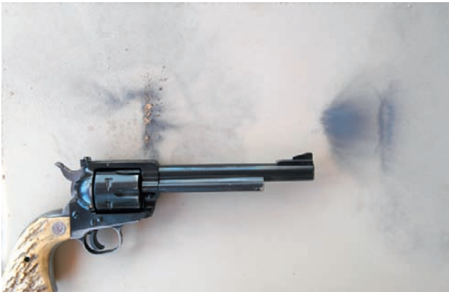
FIGURE 6.7 Muzzle and cylinder gap deposits.
