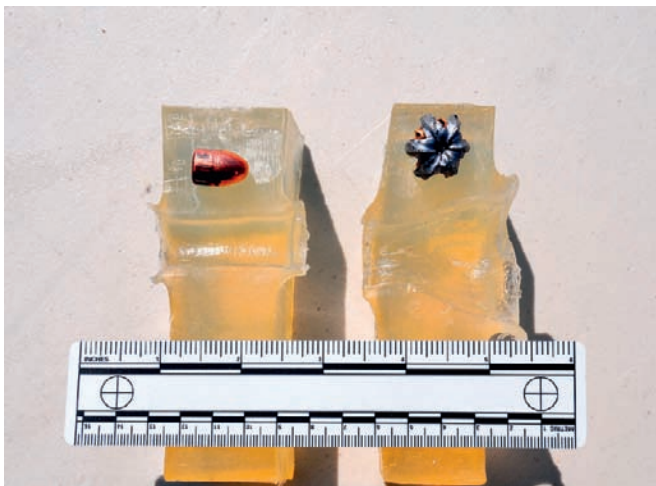
FIGURE 11.5 Both bullets perforated 1.5-inch blocks of inelastic ballistic soap from left to right as viewed. On the left, a FMJ nonexpanding bullet; on the right, an expanding hollow-point bullet.
