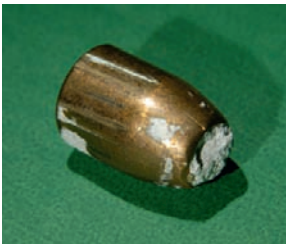
FIGURE 12.5 A bullet that perforated a panel of drywall; notice the bearing surface and nose.
