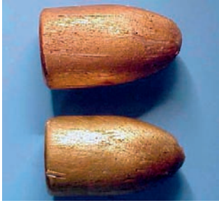
FIGURE 9.18 Two FMJ 9mm bullets ricocheted from soil.
