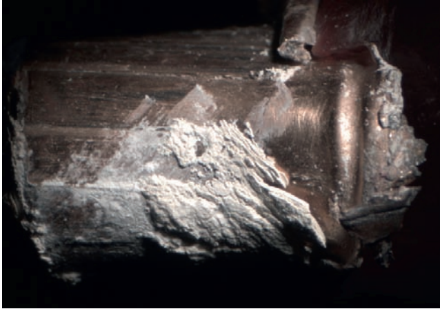
FIGURE 8.5 An unstable bullet that impacted a glass window pane. The location of the glass in the bearing surface and the size of the trace evidence tell us about the impact conditions.
