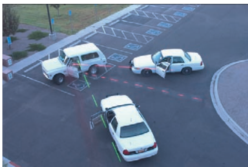
FIGURE A.9 Dotted or dashed laser lines created by moving the reflective card in and out of the laser beam intermittently as the line is walked.
