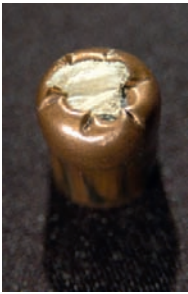
FIGURE 12.4 In this photograph, wood is trapped in a hollow-point cavity. Do not expect to see this in rifle bullets or FMJ or soft-point pistol bullets.
