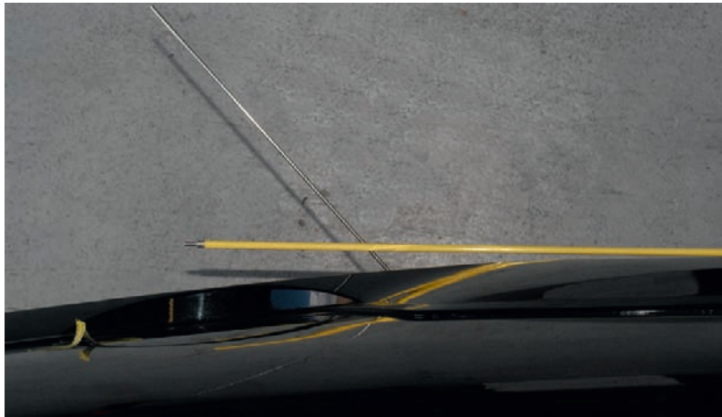
FIGURE 15.2 The yellow probe serves as a reference line, while a stainless steel rod represents the bullet's path into the vehicle.
