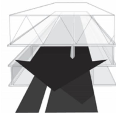
*Figure 9 Final lay out of the heat recovery roof (windbreak mesh on top not displayed)*
