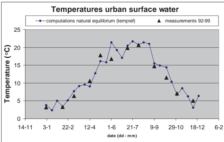
Figure 4 Natural equilibrium temperatures of a pond. LxWxD = 200x50x0.5 m. Climate conditions computations: current ('tempref' data).
