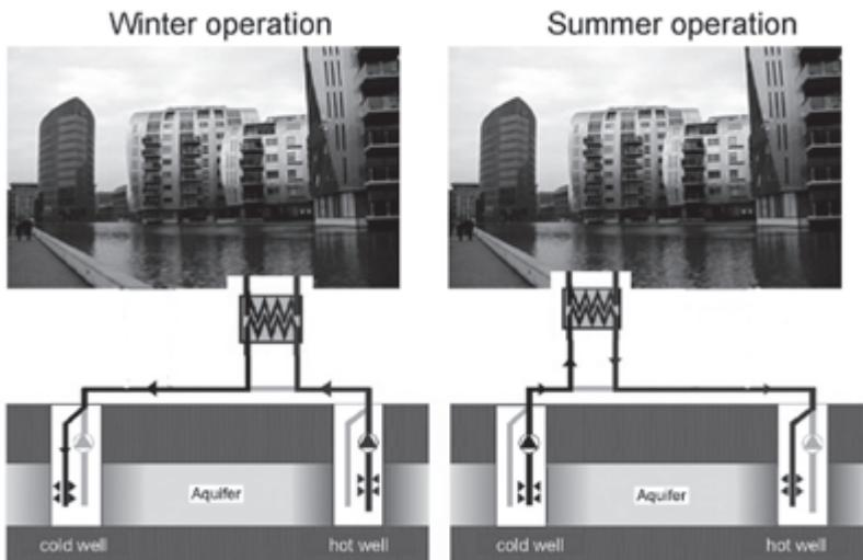
Figure 2 Energy capture using urban surface water and an aquifer
