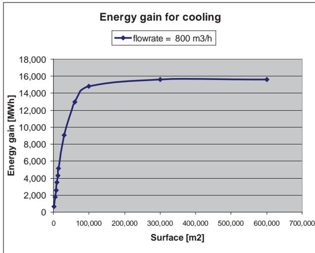
Figure 6 Energy capture potential for cooling depending on the pond surface. Depth = 0.5 m.
