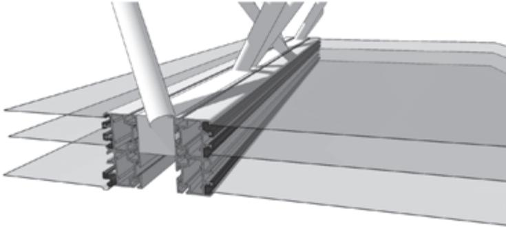
Figure 5 Membrane roof with 2 layers of 50 mm of 'standing' air,  $U_{tot} = 2.0 \text{ W/m}^2\text{K}$
