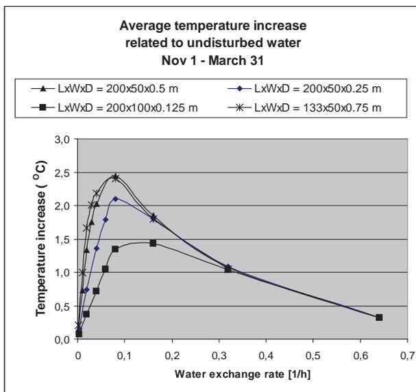
Figure 9 Temperature rise of the pond due to energy exchange with the aquifer. Climate conditions: current.
