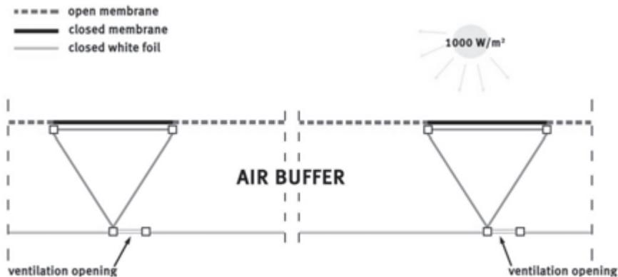
Figure 3 Detail of the roof, on top a windbreak mesh and below a semi transparent foil
