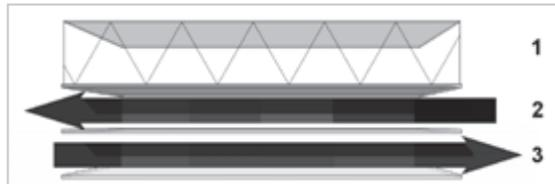
Figure 6 Concept lay up; insulation layer (1), outdoor air (2), indoor air (3) (windbreak mesh on top not displayed)
