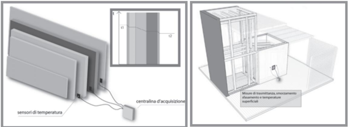
*Figures 5 and 6 Temperature values of the wall are obtained with thermometers collocated inside and on its surfaces.*
