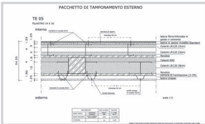
Figure 4 Technological detail of the ventilated envelope of the prototype.
