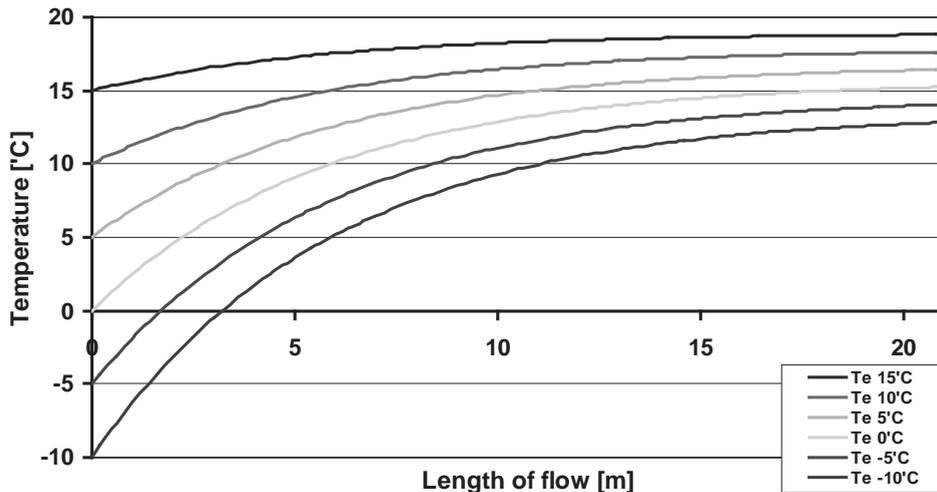
Figure 8 Results of inward flow temperatures at different outdoor temperatures ( $T_e$ ) and flow lengths
