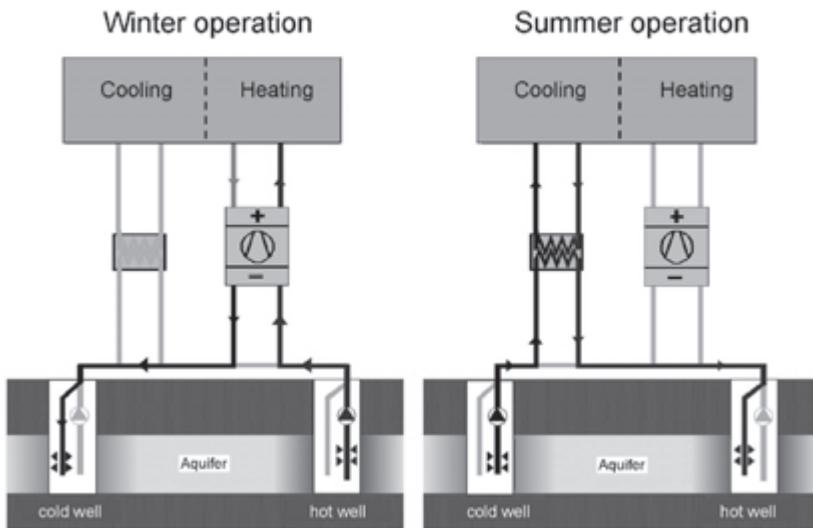
Figure 1 Energy flows due to heating and cooling by a heat pump and aquifer.
