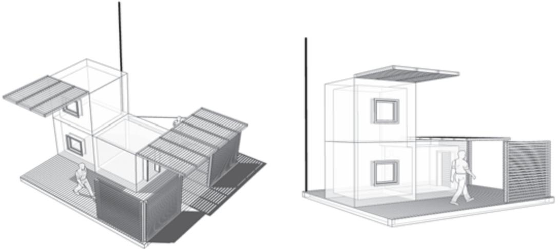
*Figures 2 and 3 Perspective views of the prototype with its mobile solar screens.*
