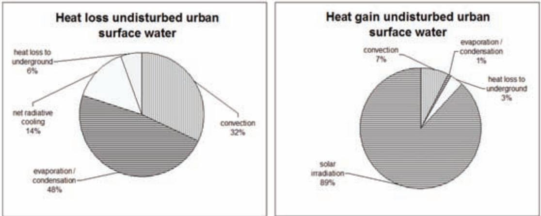
Figure 5 Energy balance of the natural dynamic equilibrium of a pond.  $L \times W \times D = 200 \times 50 \times 0.5 \text{m}$ . Climate conditions computations: current ('tempref' data).
