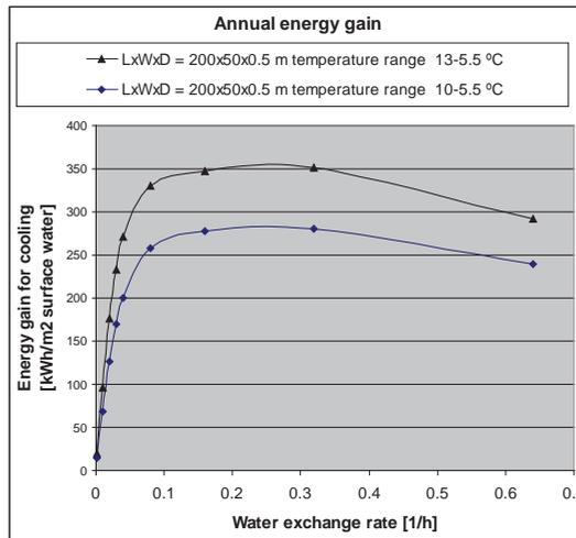
Figure 7 (top) Energy capture potential as function of the water exchange rate.
