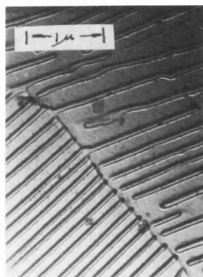
Fig. 6 Cr-V-Ni-Cu showing pearlite refinement and fine interlath carbides
