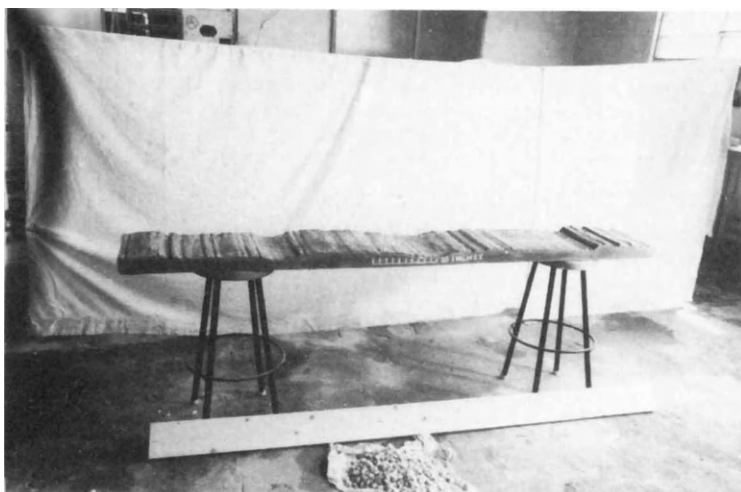
Fig.2 Model demonstration of surface texture of scaife in enlarged scale (X1000) the board represents a 2.5mm diamond and the gravel the diamond powder 2-3 \mu\text{m} .
