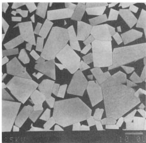
Fig. 5. Typical microstructure of a coarse straight grade cemented carbide (grey: tungsten carbide, black: cobalt). Note that both phases form a continuous network in three dimensions. (Scanning electron micrograph)
