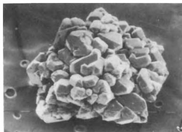
Fig. 2 A weak, intergrown polycrystal caused by interference during synthesis
