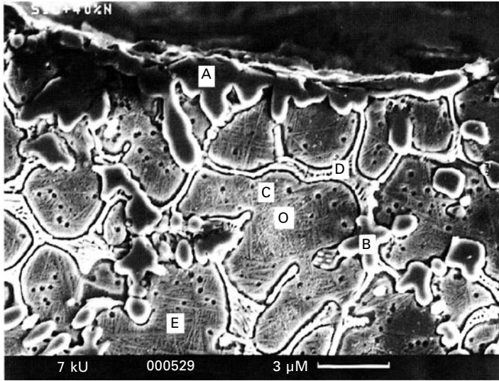
12.5 SEM micrograph showing \text{Ti}_5\text{Si}_3 particles A and B, spherical \text{TiC} in C and E, and a eutectic of \text{Ti}_5\text{Si}_3 and \alpha' -Ti, at D (Hu et al. , 1998).
