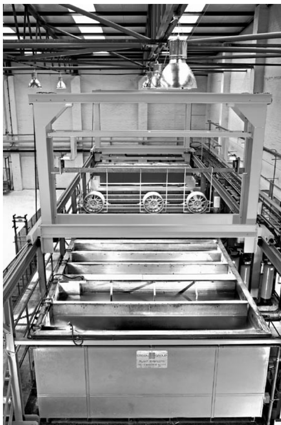
18.33 Fully automated Keronite PEO production line at Powdertech, Oxford, UK. Machine is set up for coating the three wheels shown.
