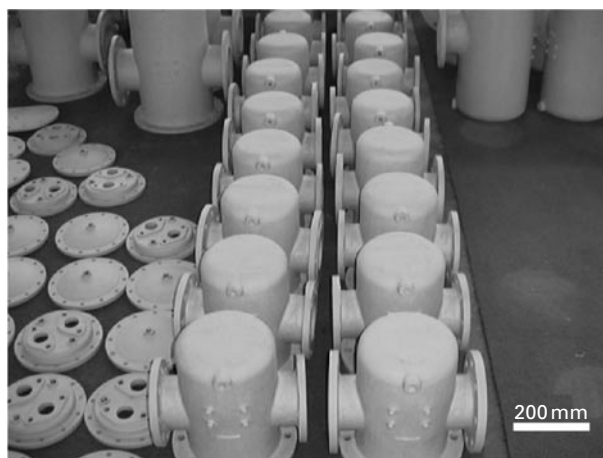
5.12 Plasma electrolytic oxidation treated seawater filtering device of ZL114 aluminium alloy for corrosion resistance.
