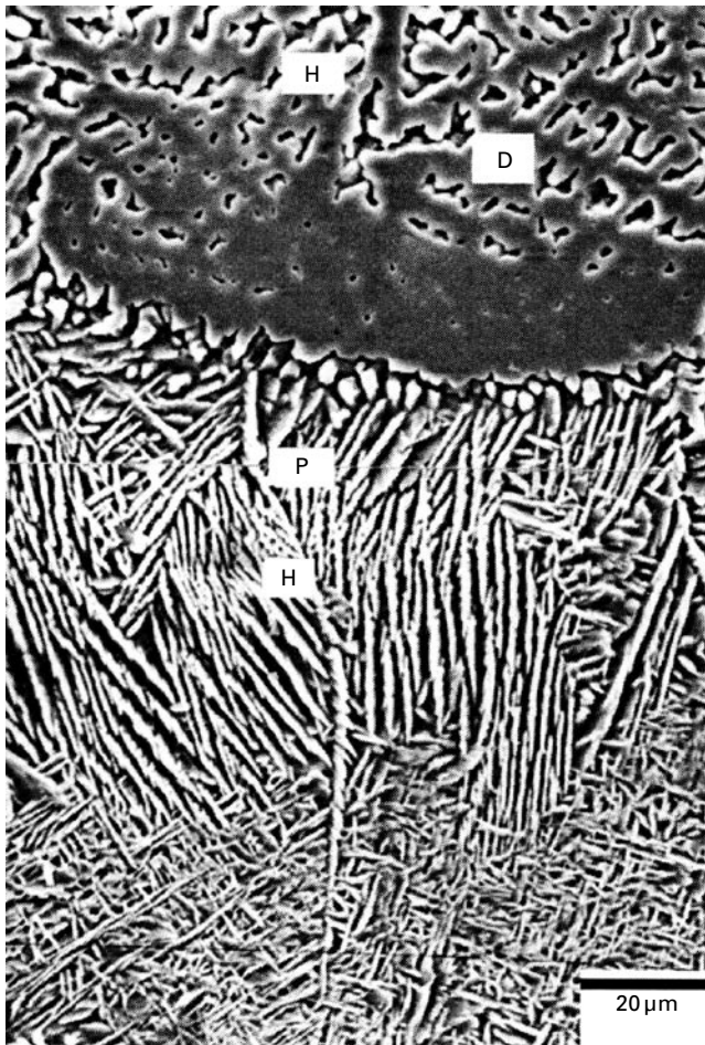
12.15 SEM micrograph of laser processed SiC preplaced powder on CPTi, showing small needles (10–15 \mu\text{m} ) below larger needles (30–35 \mu\text{m} ) following a concentrated dendritic structure (D). Platelet particles (P) in the needle structures and variation of the hardness indentations (H) are also visible (Mridha and Baker, 2007).
