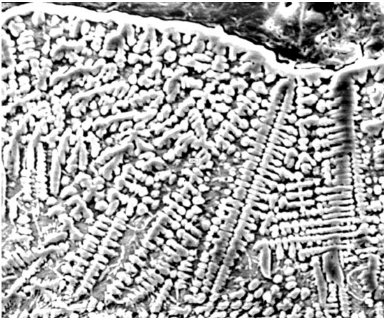
12.12 Heterogeneous distribution of dendrites following laser nitriding (Mridha and Baker, 1996).
