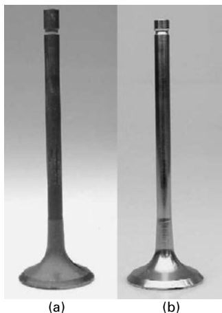
14.10 Comparison of the wear of (a) CCT and (b) PVD treated TiAl valves (Gebauer, 2006).
