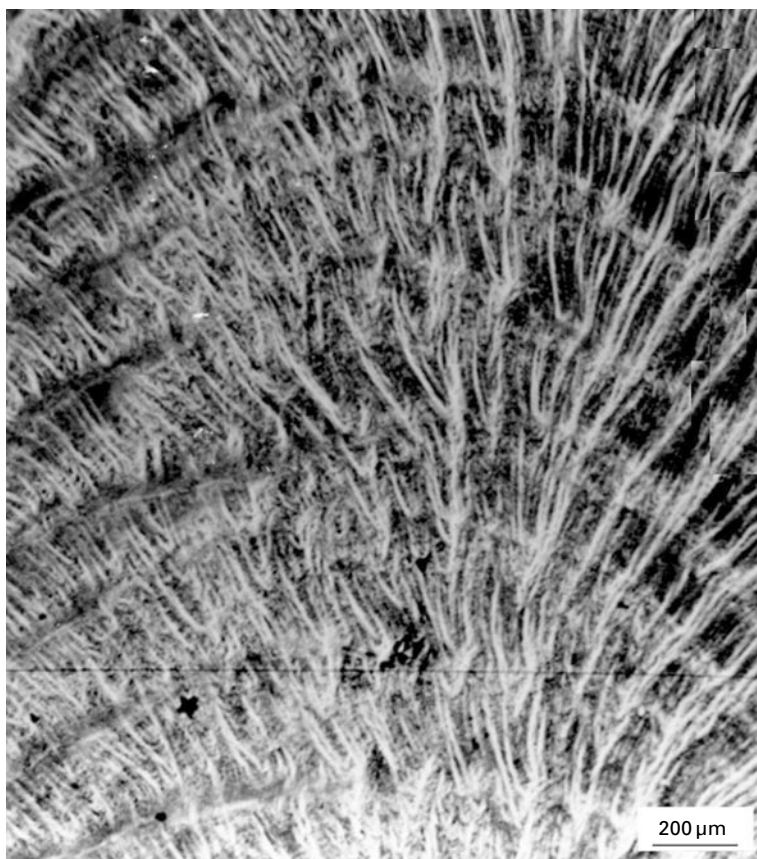
12.13 Surface topography showing rippling following laser melting of CPTi (Mridha and Baker, unpublished).
