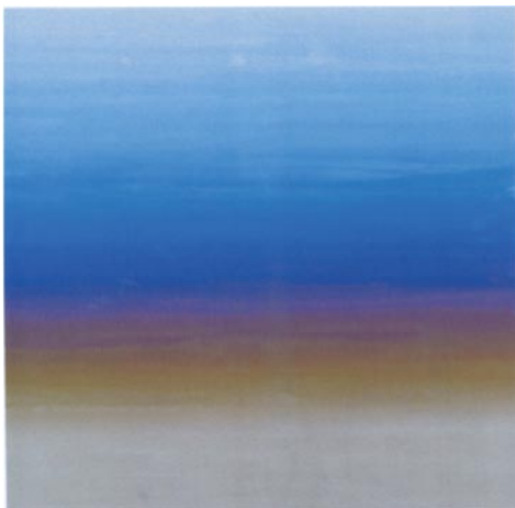
4.7 Anodised titanium, with oxide layer increasing in thickness from the bottom up (Titanium Information Group, 2006).
