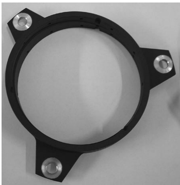
18.29 Barrel for satellites treated with new black Keronite on AA2618 alloy. The black Keronite coating has recently been extensively tested in humidity, vibration, debris formation, low optical reflectivity tests and as a sub-layer for adhesive bonding.
