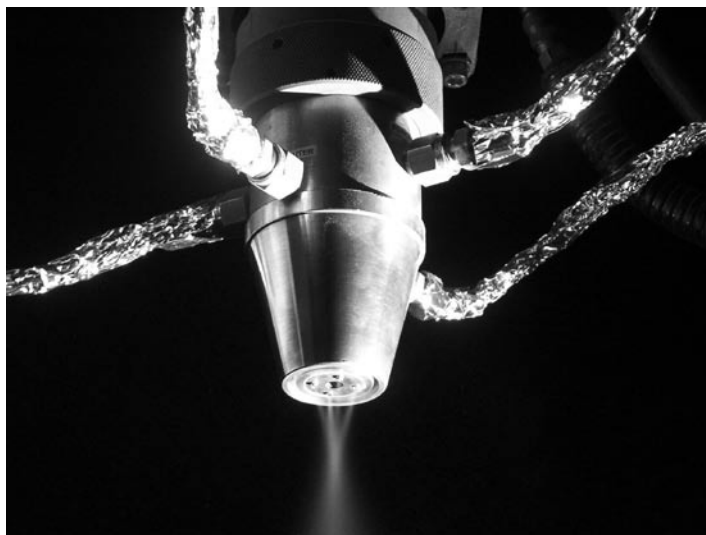
13.2 Coaxial nozzle showing flow of powder, with laser beam off.
