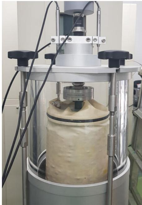
**Fig. 7.** Specimen in triaxial cell
