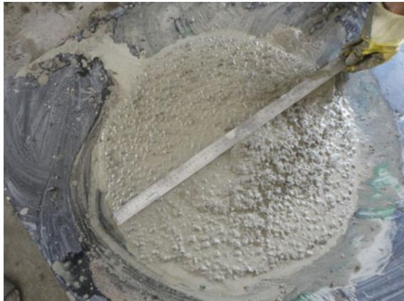
**Fig. 1.** Slump flow test for SCC mix
