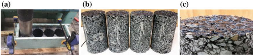
**Fig. 2.** Extraction of specimens from SBC slab: **a** coring in the frame; **b** extracted specimens with no damage; **c** close up photo of the epoxied surface
