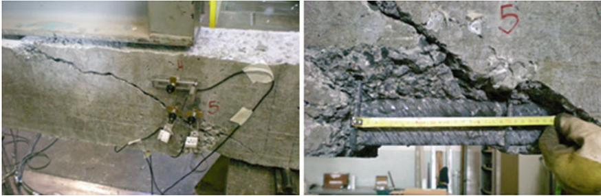
**Fig. 4.16** Shear failure in B2 beams
