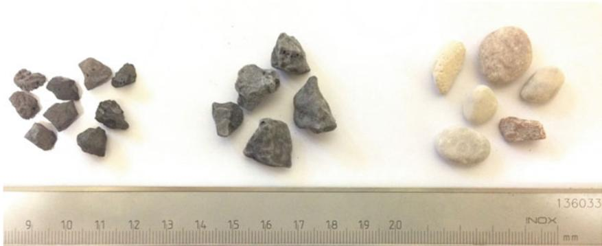
**Fig. 4.1** Electric arc furnace slag vs. siliceous aggregates
