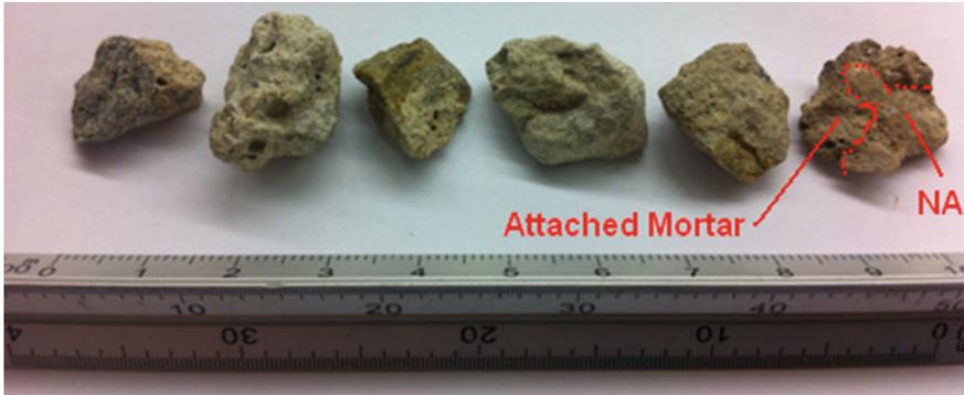
Fig. 3.12 Recycled aggregates with high attached mortar content
