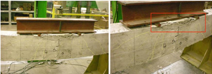
Fig. 4.12 Bending failure: concrete crushing in A2 beams
