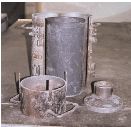
Figure 2.6. Cylindrical molds for compressive strength specimens. (IMG15523)
