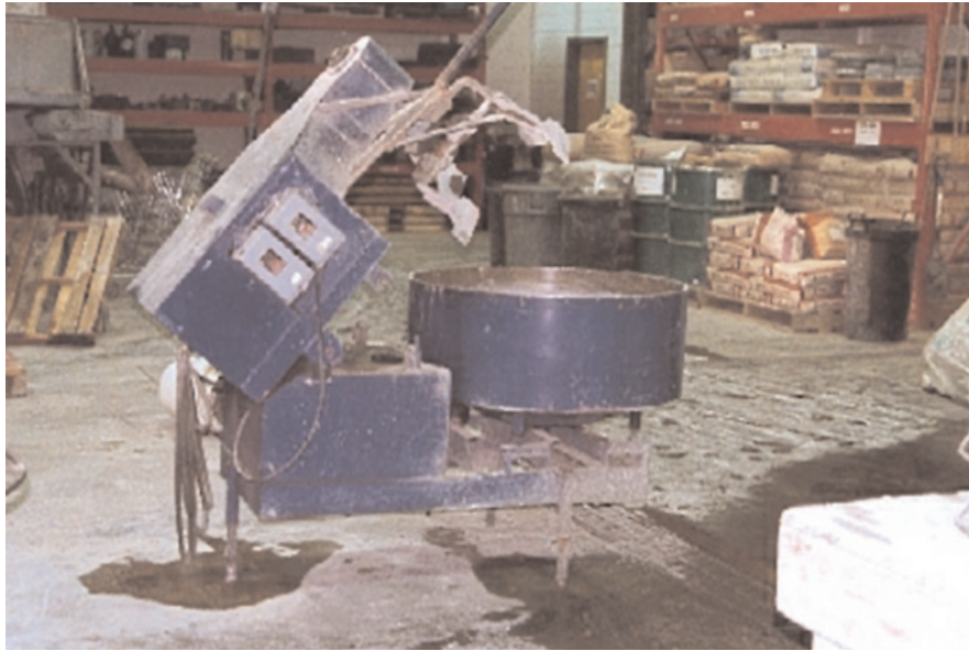
Figure 2.4. One-tenth cubic meter counter current pan mixer. (IMG15521)
