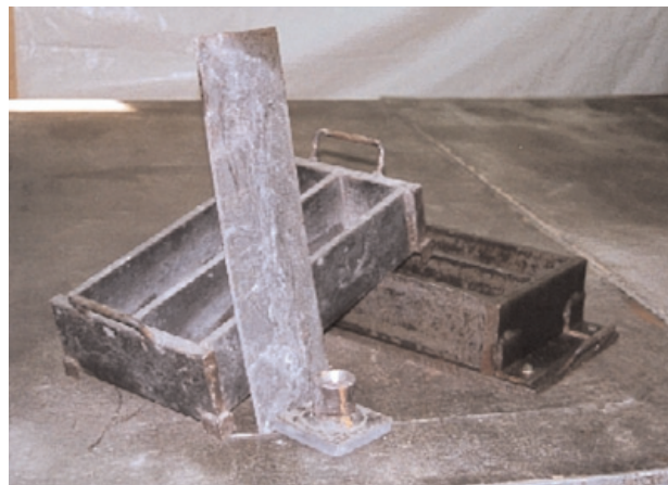
Figure 2.7. Molds used for consolidation of beams. (IMG15524)
