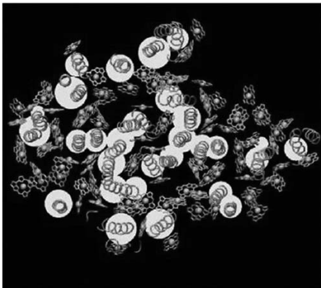
Figure 10. Dielectric model of the protein. Within this model, the protein medium (i.e., the medium with the refractive index of n = 1.2 ) is represented with a set of cylinders. The cross section of these cylinders is shown with white circles. The real location of the transmembrane part of \alpha -helices in PSI are indicated by coiled structures. Chlorophylls are presented as Mg-chlorin rings, lacking the phytol tail. Chlorophyll Mg atoms are shown in van der Waals representation. See color insert.
