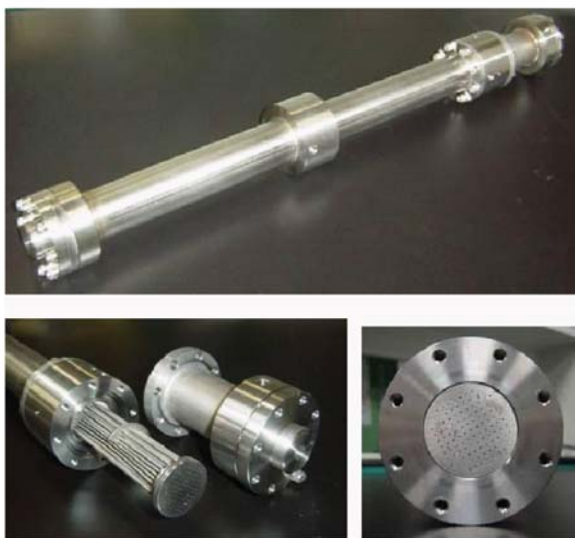
Fig. 16. a,b Two parallel microcapillary connection concepts: tube-and-shell multitubular and branched tube arrangements (Courtesy of ACS)
