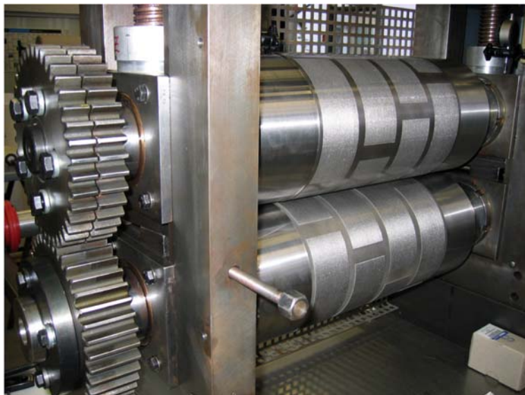
Fig. 3. Roll for mass fabrication of microstructured steel plates. The endless sheet can be moved at least at a velocity of 1 m/min, i.e., for a plate length of 10 cm and rolling four microstructured units in parallel, 2,400 plates/h can be manufactured. Structural dimensions of 500 \mu\text{m} have so far been realized; the technique is expected to yield microstructures at a 100- \mu\text{m} characteristic width
