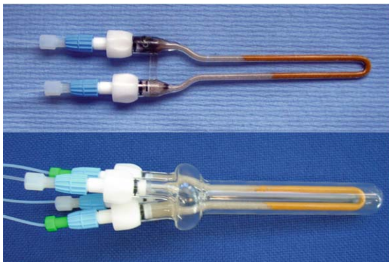
Fig. 10. Pd EnCat microwave reactor columns, simple U-tube and enclosed system
