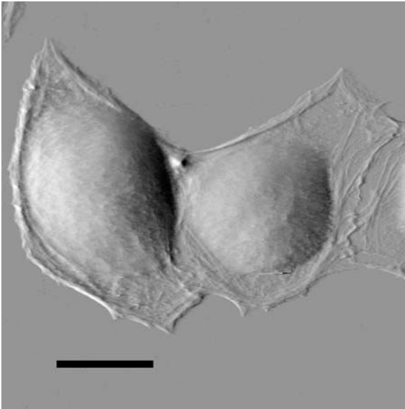
Atomic Force Microscopy. Figure 2 An AFM contact-mode image of conjoined NRK daughter cells. The image was recorded about 30 min after cytokinesis. Dynamically and spatially-resolved changes in cortical stiffness that play a role in cell division can be observed with the force microscope. Scale bar 20 \mu\text{m} . (From: Matzke R, Jacobson K and Radmacher M (2001) Direct, high-resolution measurement of furrow stiffening during division of adherent cells. Nat Cell Biol 3:607–610).
