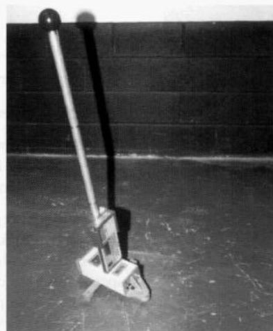
(b) Dipstick for measuring Properties I and II.
