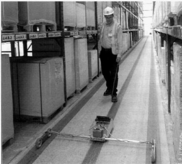
Figure 4.8: Profileograph in use in an aisle.
