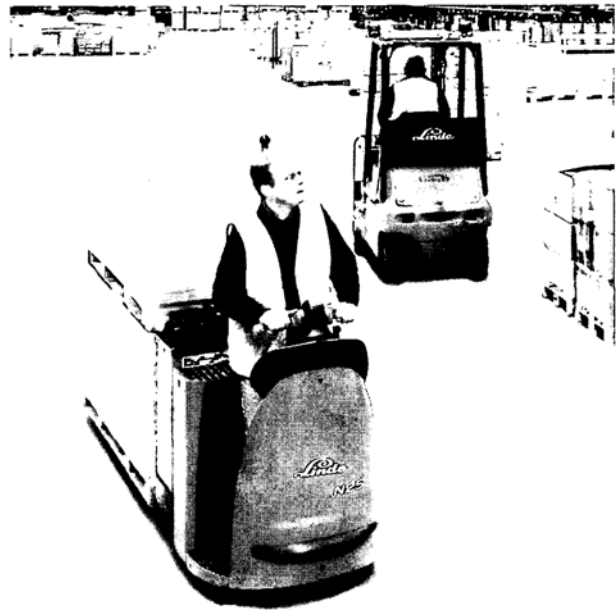
Figure 3.13: The small wheels on pallet trucks (such as that in the foreground) can be damaging to joints in floors.
