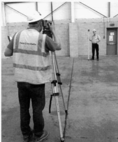
(a) Optical level for measuring Property IV and datum.
