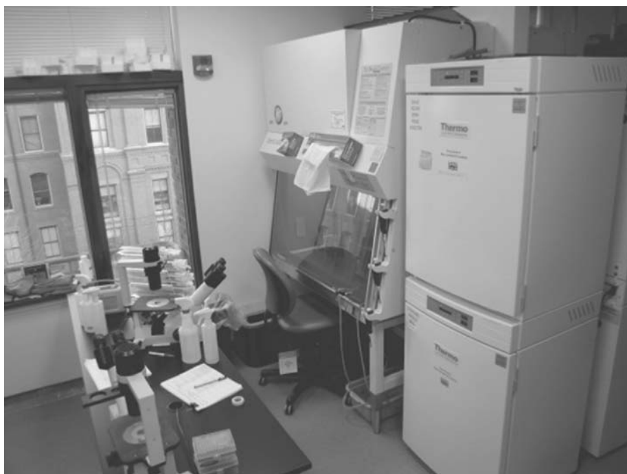
Figure 1 Typical biosafety cabinet set up. The cabinet is organized so that the user work space is uncluttered while items such as pipettes, tissue paper for cleaning, waste containers, etc. are all close to hand.
