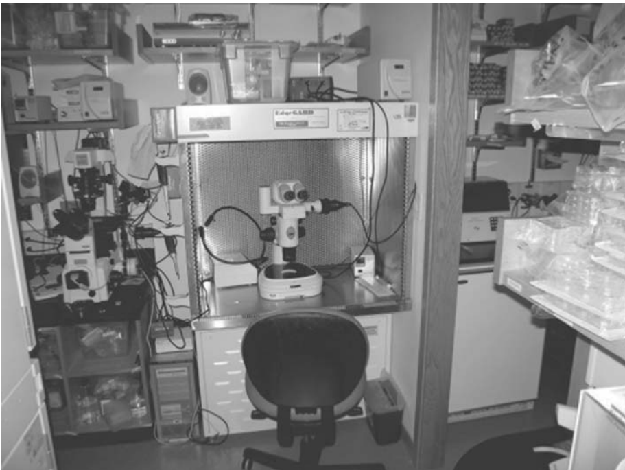
Figure 2 Typical embryo manipulation set up. A dissection microscope with heated stage is positioned in a laminar air hood to minimize the risk of microbial contamination while working.
