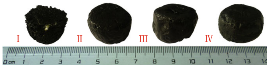
Fig. 4.2 Photographs of the as-prepared (I) G–S mix using GO and sulfur as precursors and (II)–(IV) G–S hybrids using GO, sulfur-dissolving CS 2 , and alcohol dispersion as precursors, after hydrothermal treatment at 180 °C for 10 h
