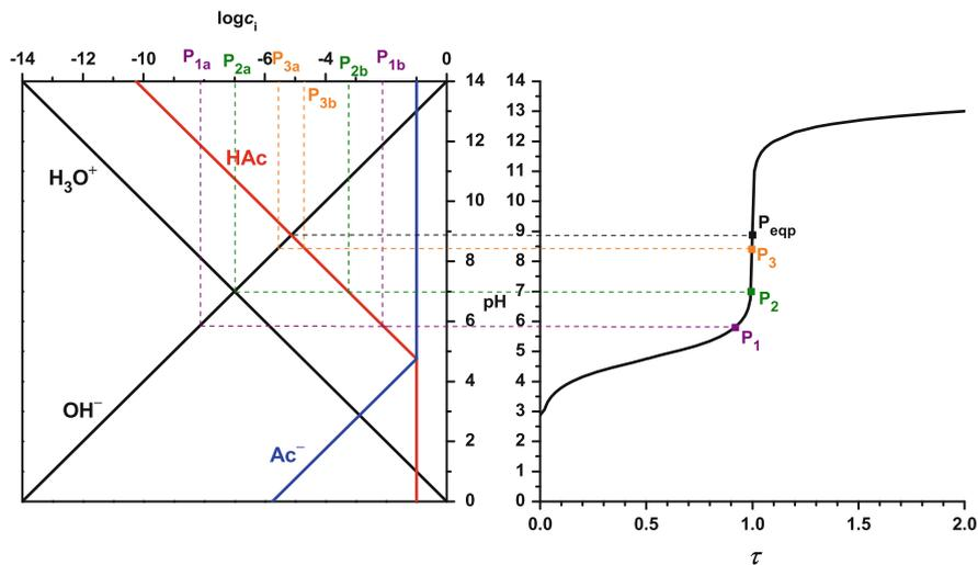
**Fig. 84** Reading of the relevant concentration data from the  $\text{pH}-\log c_i$  diagram for estimation of the systematic titration errors in case of the titration of acetic acid ( $C_{\text{acetic acid}}^{\circ} = 0.1 \text{ mol L}^{-1}$ ) with sodium hydroxide.  $P_{\text{eq}}$ : equivalence point,  $P_1$  to  $P_3$  are transition points of the indicators methyl red, neutral red, and phenolphthalein
