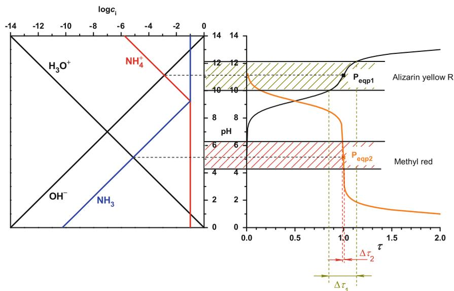
**Fig. 88** pH- $\log c_i$  diagram and diagram of the titrations of ammonia with hydrochloric acid (orange line with equivalence point  $P_{\text{eqp2}}$ ) and of ammonium ions with sodium hydroxide (black line with equivalence point  $P_{\text{eqp1}}$ ). The shadowed ranges indicate the transition ranges of the indicators alizarin yellow R and methyl red
