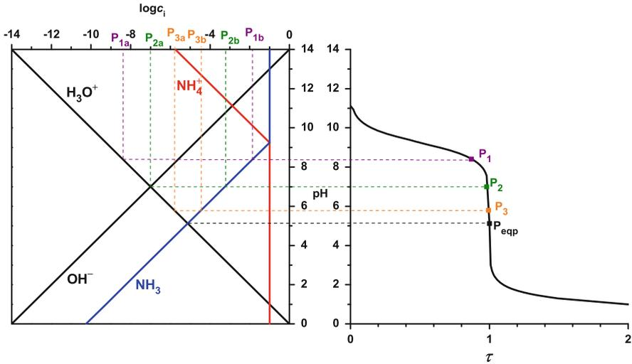
**Fig. 85** Reading of the relevant concentration data from the pH- $\log c_i$  diagram for estimation of the systematic titration errors in case of the titration of ammonia ( $C_{\text{ammonia}}^{\circ} = 0.1 \text{ mol L}^{-1}$ ) with hydrochloric acid using different color indicators:  $P_{\text{eq}}$ : equivalence point,  $P_1$  to  $P_3$  are the transition points of the indicators phenolphthalein, neutral red, and methyl red
