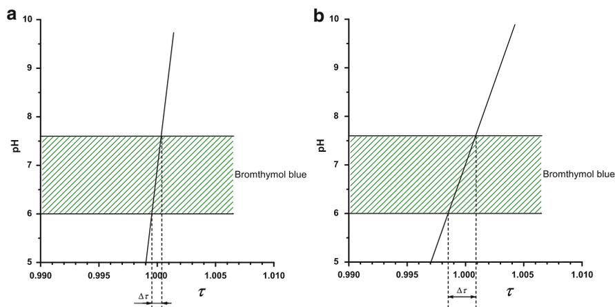
**Fig. 87**  $\Delta\tau$  range corresponding to a fixed pH range of the transition of an indicator (here bromthymol blue; transition range from pH 6.0 to 7.7): (a) for the case of a titration curve which is very steep in that pH range, and (b) for a titration curve which is less steep in that range
