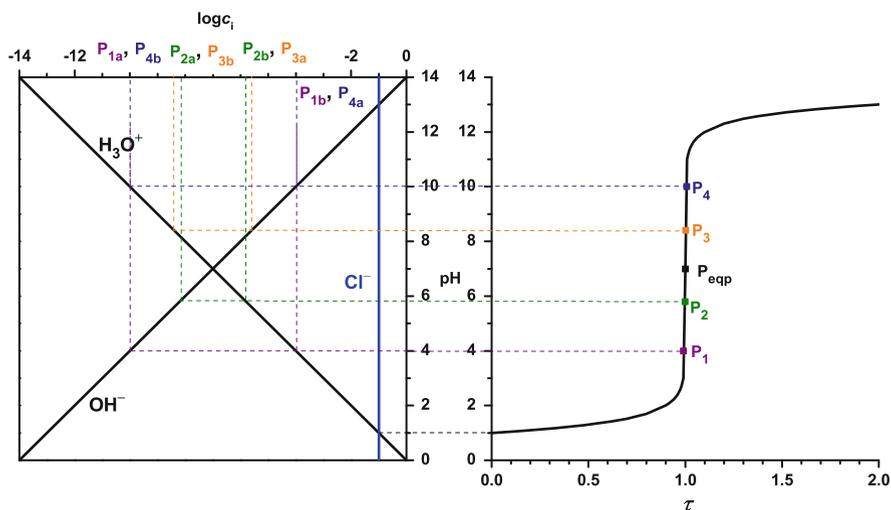
**Fig. 86** Reading of the relevant concentration data from the pH- $\log c_i$  diagram for estimation of the systematic titration errors in case of the titration of hydrochloric acid ( $C_{\text{hydrochloric acid}}^{\circ} = 0.1 \text{ mol L}^{-1}$ ) with sodium hydroxide.  $P_{\text{eqp}}$ : equivalence point,  $P_1$  to  $P_4$  are the transition points of the color indicators methyl orange, methyl red, phenolphthalein, and thymolphthalein
