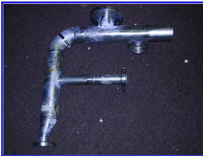
*Figure 5. Pipe in >95% HNO<sub>3</sub> 50 °C Service. Note the corroded areas are less extensive. (see color insert)*
