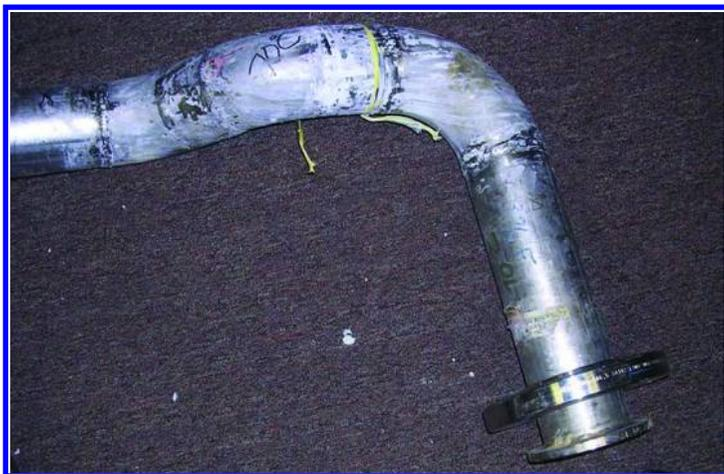
*Figure 4. Pipe in >95% HNO<sub>3</sub> 70 °C Service. Corrosion is seen in between and along welds (white area). (see color insert)*
