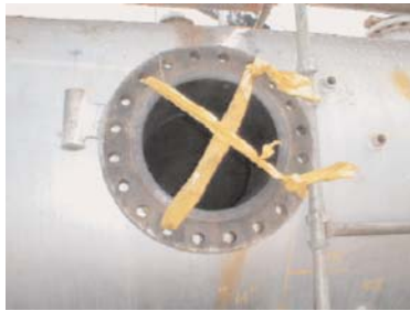
Picture of the separator after the incident, with inadequate physical barrier and lack of signage.
