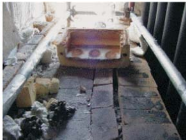
Burner tile on reformer floor 18 ft (5.5 m) below
