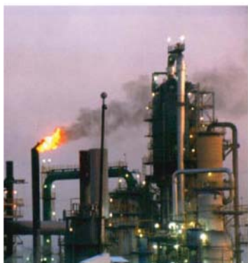
Figure 61 Flames coming out of stacks of fired heaters after tube ruptures.
