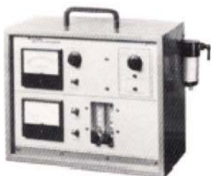
Figure 12 These analysers measure the amount of oxygen and combustibles present in flue gas.
