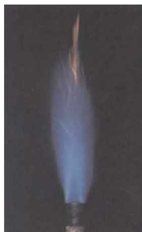
Figure 35b Good pilot flame.
