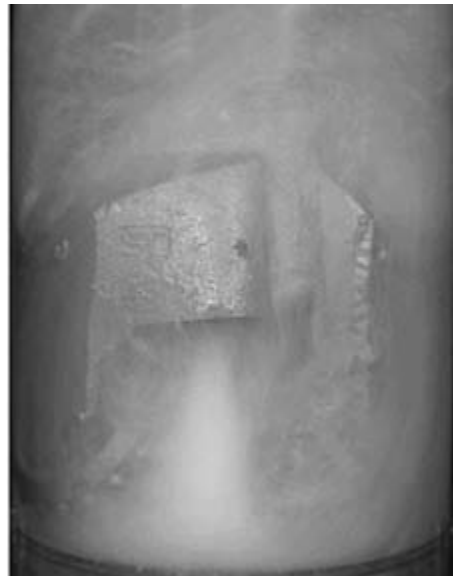
Figure 4.7.4 Hydraulic flow around bit body.
