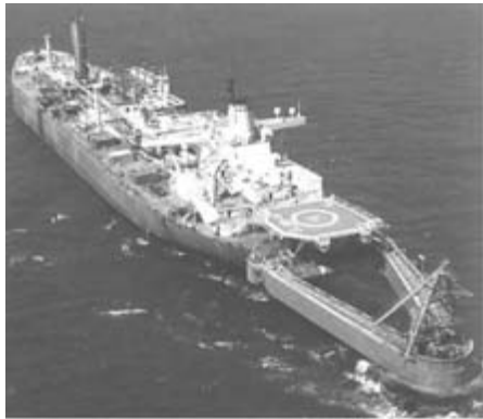
Figure 6.10.8 Externally mounted SPM on FPSO Buffalo Venture [ http://www.offshore-technology.com/project/marlim/ ].
