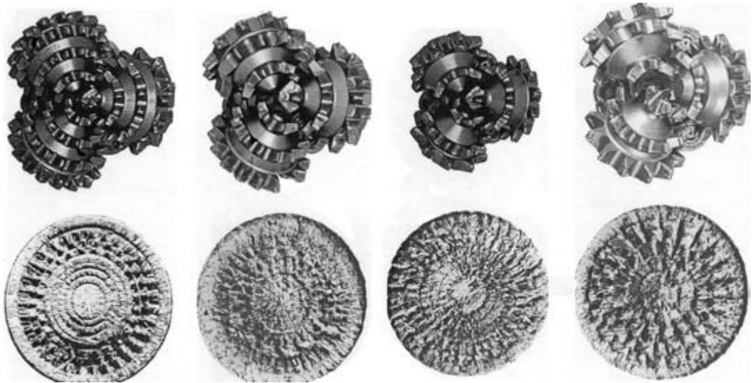
Figure 4.7.27 Soft and hard formation cutting structures.
