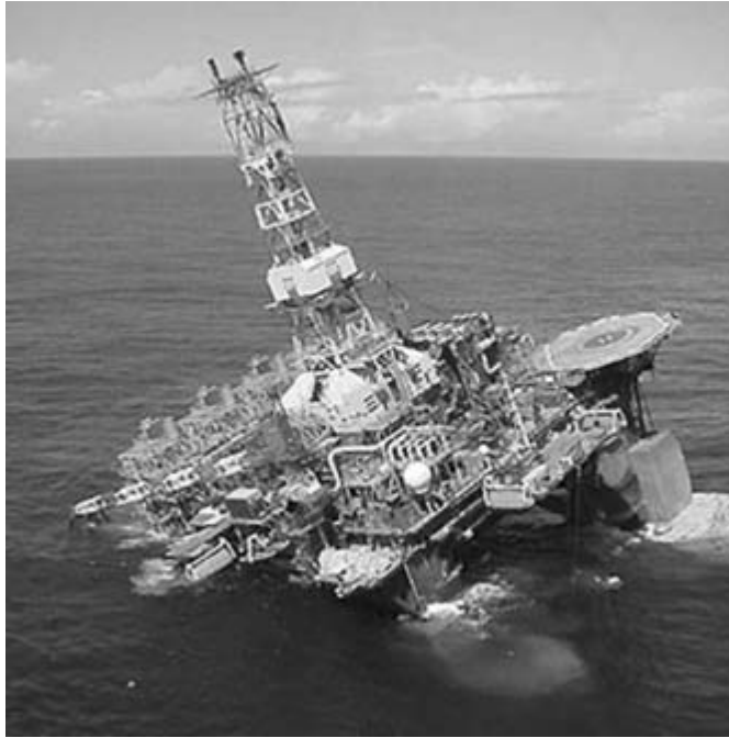
Figure 6.10.9 P-36 semi-submersible shortly before it submerged offshore Brazil [ http://www.offshore-technology.com/projects/roncador/ ].
