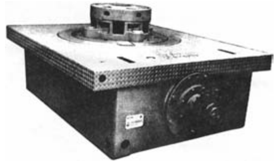
Figure 4.3.13 Rotary table with pin drive master bushings.
