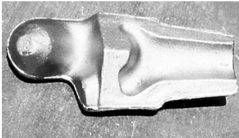
Figure 4.7.19 Roller cone bit leg forging (three required).
