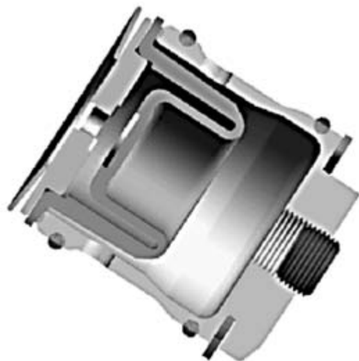
Figure 4.7.45 Typical roller cone bit lubricant reservoir.
