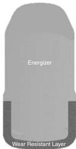
Figure 4.7.43 Cross-section of modern bi-material seal.
