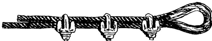
Figure 4.2.68 Correct method of attaching clips to wire rope [3].
