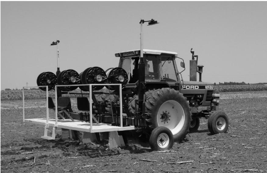
Figure 13.21. Tractor-drawn SDI installation implement installing dripline in Kansas. Courtesy of F. R. Lamm, Kansas State University.
