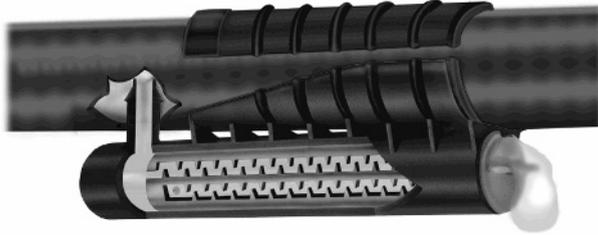
Figure 12.2. Schematic of a turbulent-flow, tortuous-path drip emitter. Courtesy of Bowsmith, Inc.
