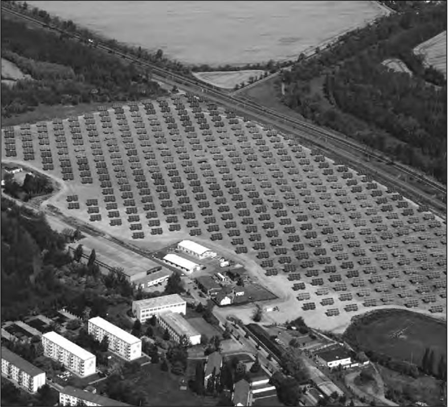
In 2006, a 3.44MWp solar array was installed on the grounds of a former coal briquette plant in Borna
