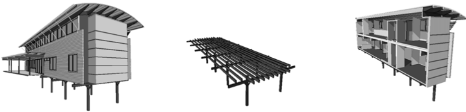
Fig. 1.15 Example of a timber block construction that can be dismantled
