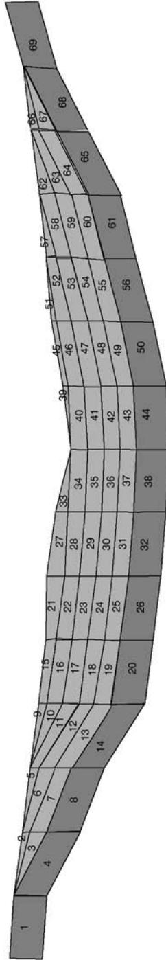
Figure 8.11 QUAD4 FEM scheme of a valley.
