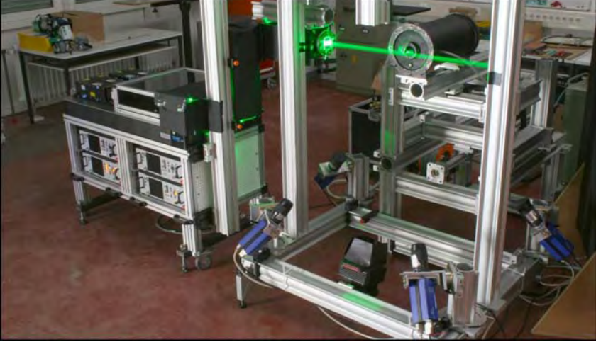
Fig. 4 Arrangement of the four pco.2000 cameras mounted under Scheimpflug-condition below the nozzle. The Big Sky CFR 200 laser system on the left illuminates the measurement volume in front of the nozzle
