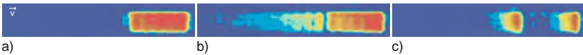
Fig. 2 Intensity response for rectangles, moving from left to right. Three cases are shown for different velocities v in relation to the system time constant \tau for objects of length l . a) v/l \gg 1/\tau , b) v/l \approx 1/\tau , c) v/l \ll 1/\tau
