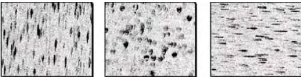
Fig. 2 Dependence of the particle image shape on the position in the measurement volume (only a thin sheet in the measurement volume is illuminated)
