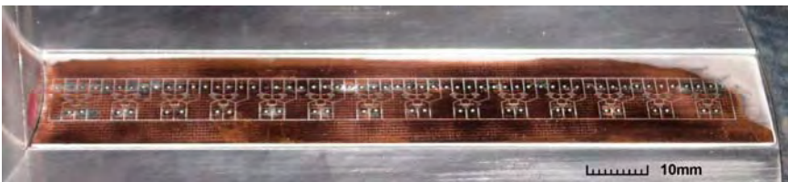
Fig. 5 Linear array of 14 delta surface hot-wire probes on the turntable
