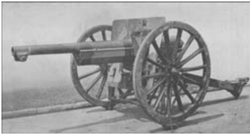
Figure 7.2 A French 75-mm gun and carriage. From U.S. Ordnance Department, Handbook of Artillery , 75.
