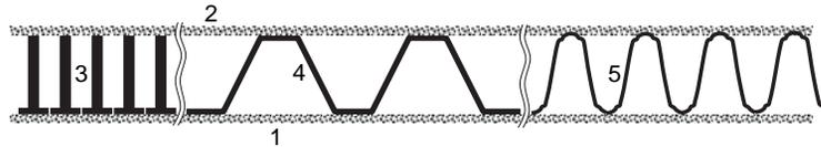
Core designs other than those shown here are also used. The purpose of the core is to support the geotextile membrane without hindering the flow of water within the thickness of the geosynthetic.
