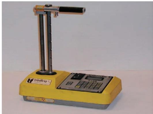
**Fig. 3.1** An example of equipment where the neutron scattering method is combined with the gamma ray attenuation method is this Troxler instrument. Courtesy of the Danish Road Institute
