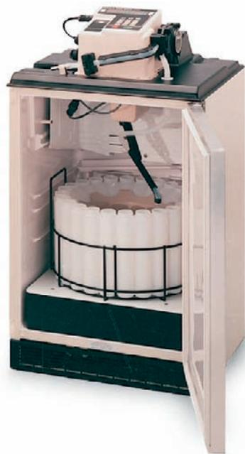
**Fig. 7.3** Automatic water sampler with refrigerated cabinet (Courtesy of Hach. ©Hach Company, 2007)
