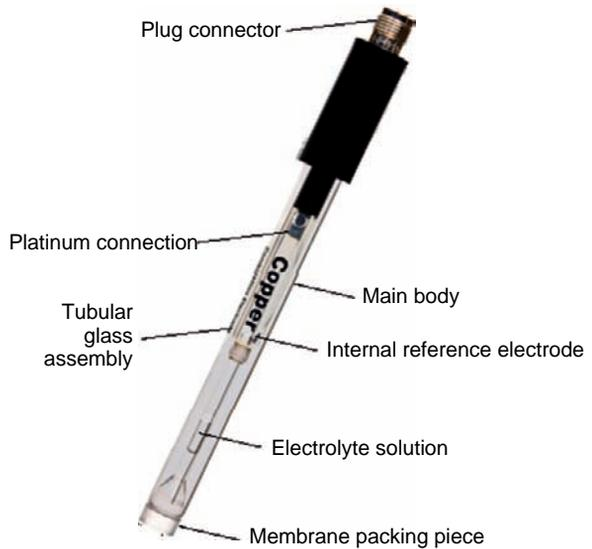
**Fig. 7.12** Ion selective electrode (Medek, 1993, Zýka, 1991). In this version, adapted from, and reproduced by permission of van London – pHoenix company
