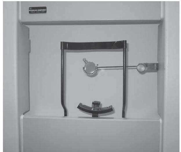
Fig. 6. Patient's end of machine showing a view through chin rest with lens holder in position. The small fixation spot is visible just right of the lens.
