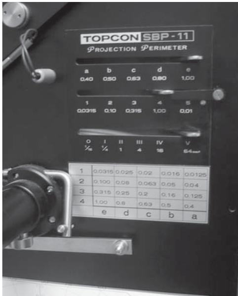
Fig. 3. Close-up from Fig. 2 showing levers for target selection. The levers are set for a V4e target. Note the chart indicating the brightness for various letter and arabic numeral lever combinations, measured in thousands of apostilbs (i.e., 4e = 1.00 = 1000 asb). The area ( $\text{mm}^2$ ) of each target size designated by Roman numerals is also shown under the lowest lever (see Table 2).
