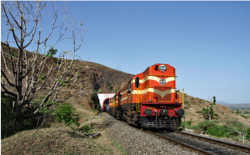
Fig. 4 WDM3A class locomotives with high-adhesion bogies for heavy freight operations
