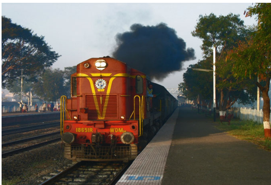
Fig. 3 A WDM2 rebuilt as 3100 hp WDM3A by DMW patiala
