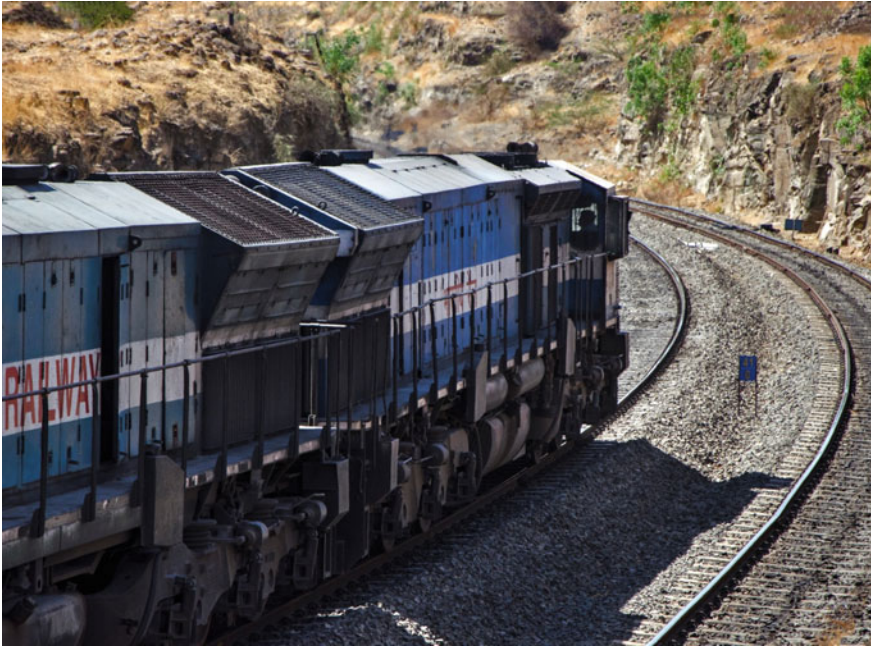
Fig. 8 Radiator compartments on the WDP4 class EMD locomotives
