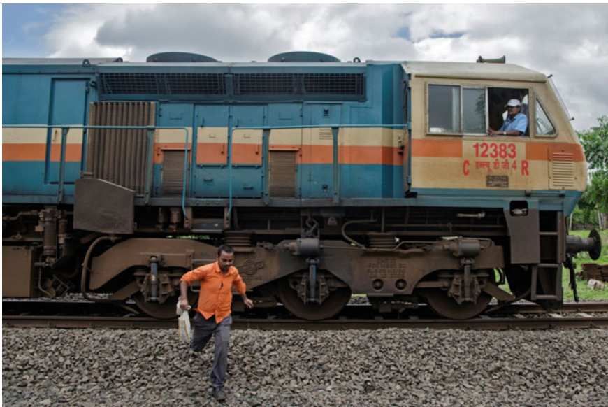
Fig. 7 HTSC bogies on the WDG4 and dynamic braking grids and fans
