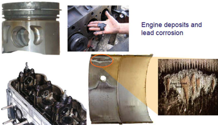
Fig. 23 Effect of biodiesel on conventional diesel engine oils [9]
