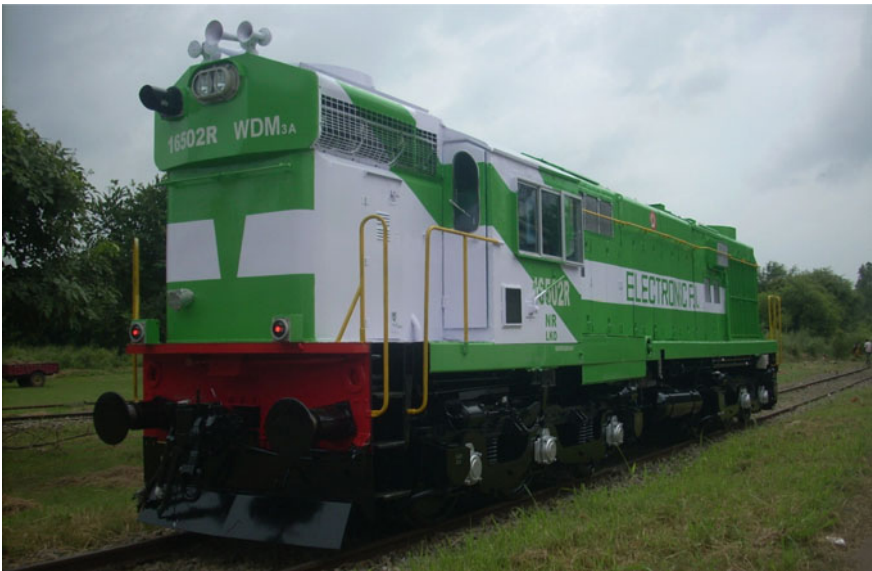
Fig. 6 A short-hood view of the EFI locomotive (Photo courtesy: Prof. Avinash K. Agarwal)
