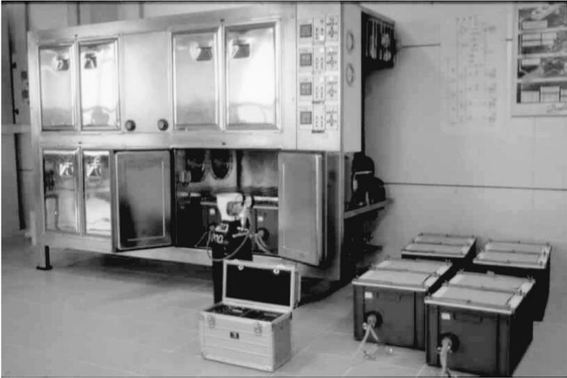
**Figure 6.3** Closed boxes used to control the relative humidity and atmosphere ( $O_2$  and  $CO_2$ ) in hazelnut cold storage studies.
