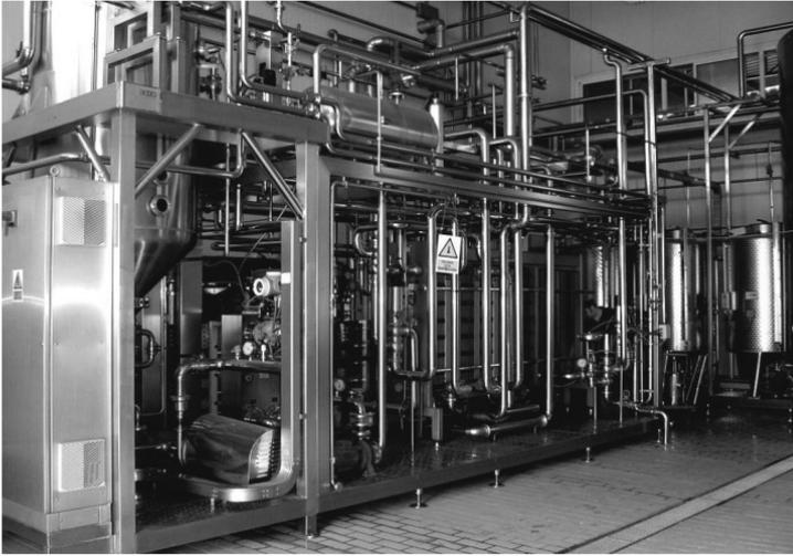
**Figure 8.17** An external hygienic design of food processing equipment.
