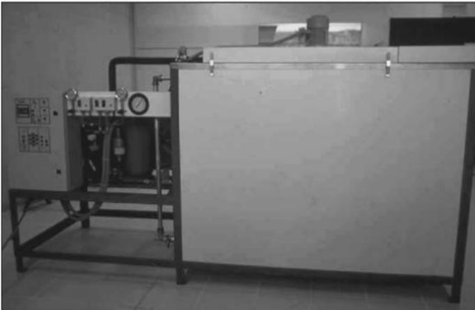
**Figure 2.20** Ice-on-coil storage system at pilot plant scale.
