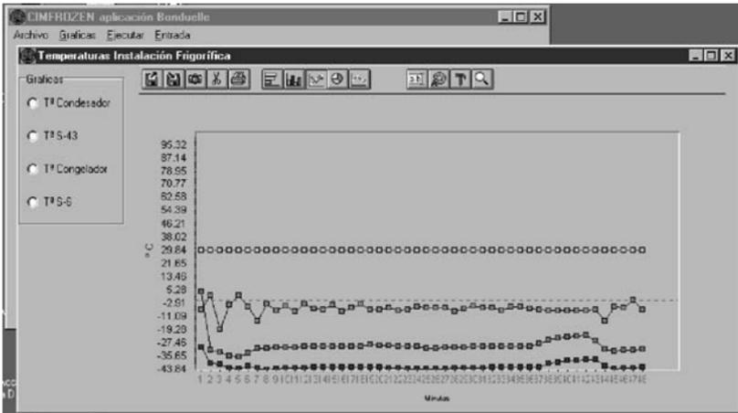
**Figure 2.34** Window showing graphics obtained from freezers and refrigeration system simulation (adapted from López et al., 1998).
