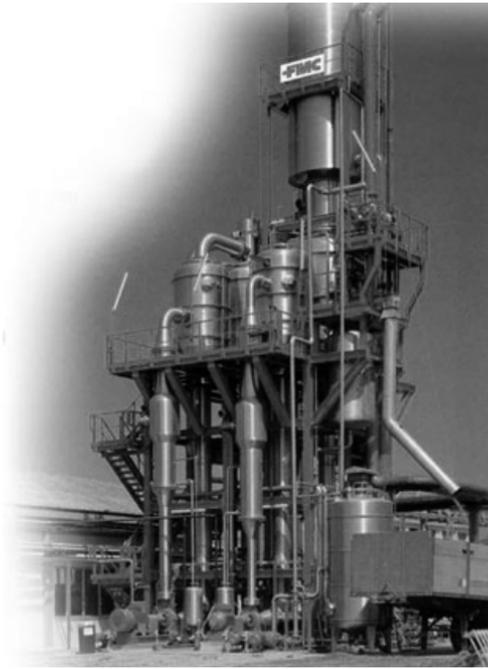
**Figure 1.4** Evaporator for concentration of juices (courtesy of FMC Food Tech, Chicago, Ill.).
