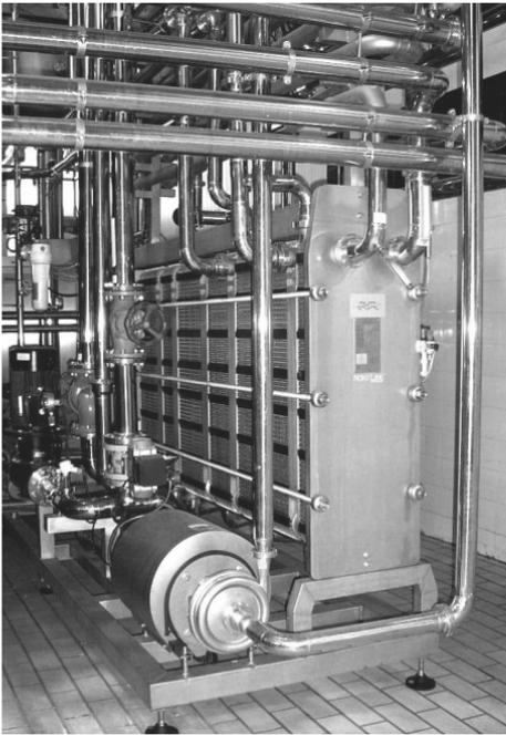
**Figure 8.8** Engine pump group with sanitary centrifugal pump and engine lined with stainless steel sheets.
