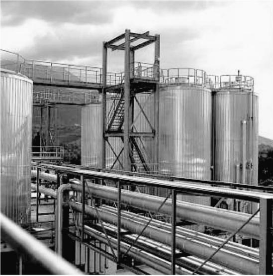
**Figure 7.2** Beer-making installation. Material in contact with the must and beer is stainless steel (courtesy of Dizio, [www.dizio.it](http://www.dizio.it)).
