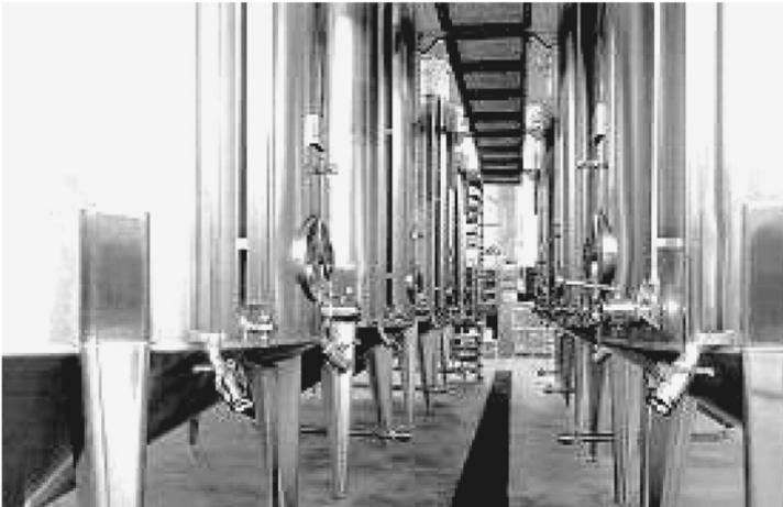
**Figure 7.3** AISI 304 stainless steel is the most widely used construction material in the food industry. In this photo, AISI 304 is used for the tanks (courtesy of Dizio, [www.dizio.it](http://www.dizio.it)).
