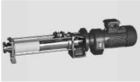
**Figure 8.6** Positive displacement rotary pump with screw rotor, constructed in stainless steel and stator in plastic material (courtesy of Alfa Laval, [www.alfalaval.com](http://www.alfalaval.com)).
