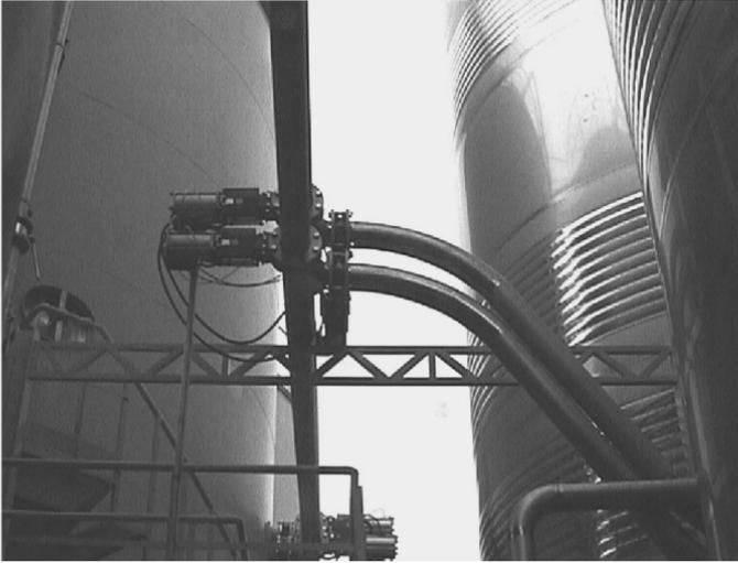
**Figure 1.9** System for transporting crushed grapes into fermentation tanks.
