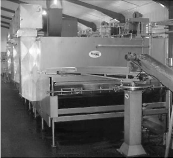
**Figure 6.1** Single-stage dryer plant (courtesy of the National Drying Machinery Company, Aeroglide Corp., [www.nationaldrying.com](http://www.nationaldrying.com)).
