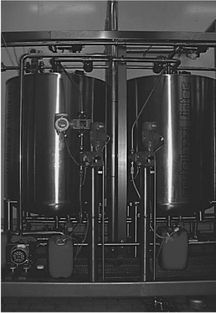
**Figure 8.24** Multitank CIP system with concentration control instruments (by conductivity) and dosage-pumps to control the reposition of cleaning products.
