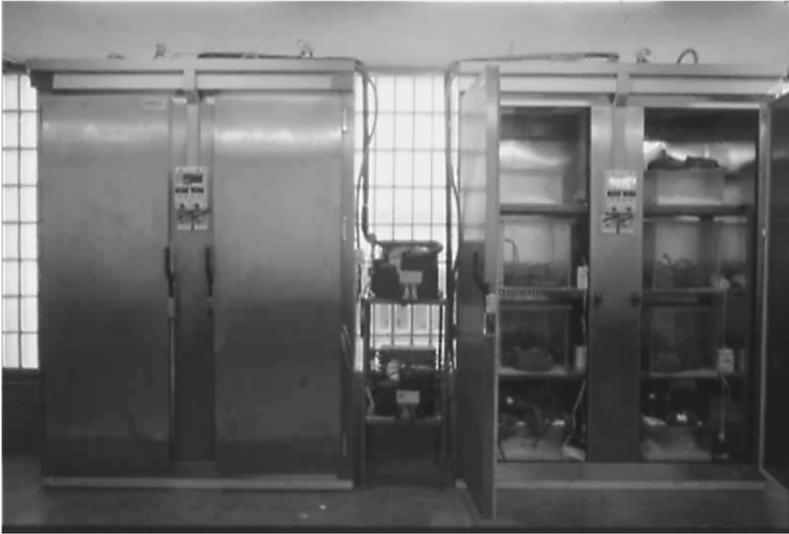
**Figure 6.2** Pilot plant or experimental installation to study the influence of cold storage conditions on hazelnut quality.
