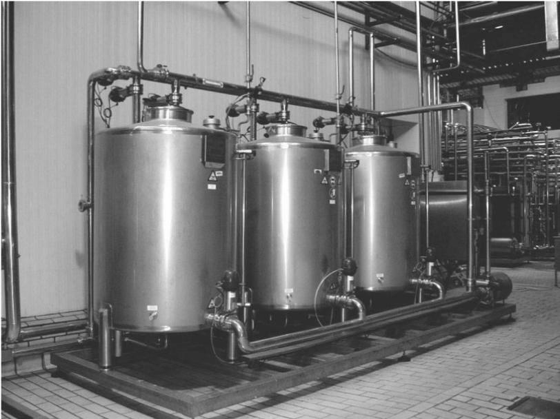
**Figure 8.22** Multitank CIP system.
