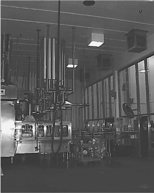
**Figure 9.1** In a citrus juice factory, the juice packaging room is a separate zone that is overpressurized with filtered air.
