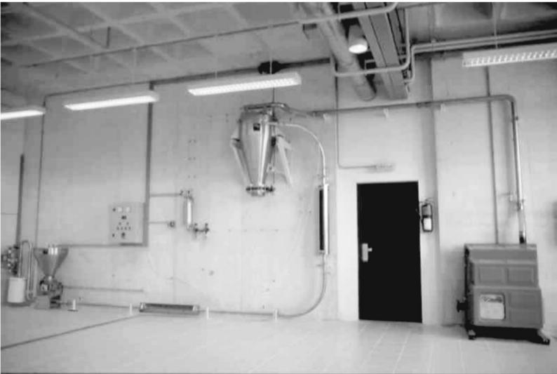
**Figure 6.5** An experimental installation to study the pneumatic transport of powder products.
