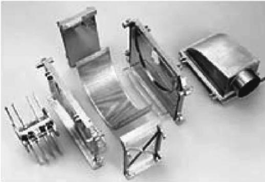
**Figure 8.1** Readily disassembled mill for inspection, cleaning, and sanitizing (courtesy of Fitzpatrick Co., [www.fitzmill.com](http://www.fitzmill.com)).
