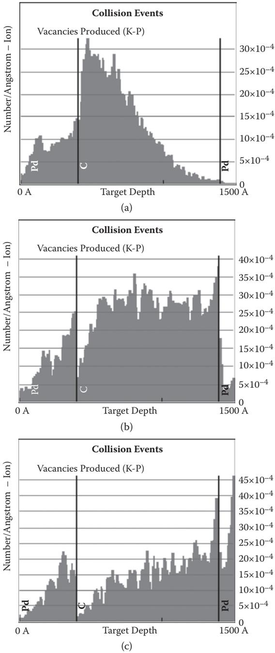
**FIGURE 3.2** Trend of collision events using SRIM 2008. (a) 5 keV, (b) 10 keV, (c) 20 keV.
